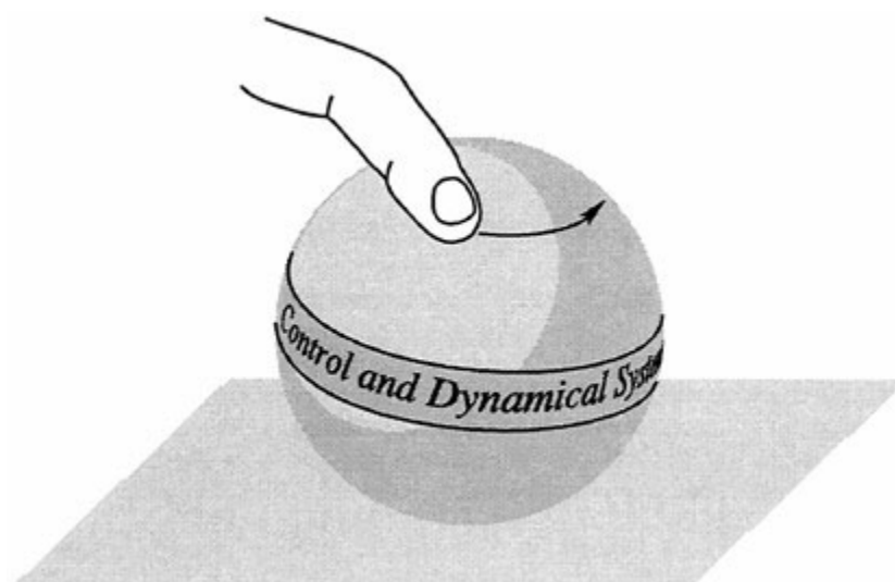
FIGURE 1.2 Rolling your finger in a circular motion on a rolling sphere generates rotations.
