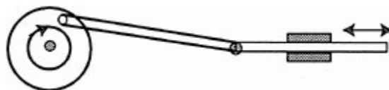
FIGURE 2.5 Converting rotary to reciprocating motion.
