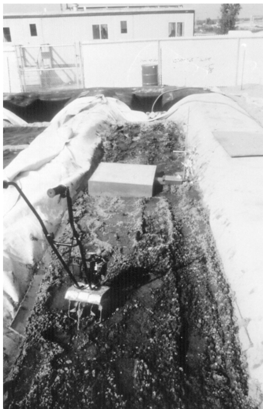
Pilot-scale land biotreatment units used to assess biotransformation and biodegradation of PCB-contaminated sediment and sludge. Pilot-scale tests are needed to assess practical treatment rates. Courtesy of Alcoa.
