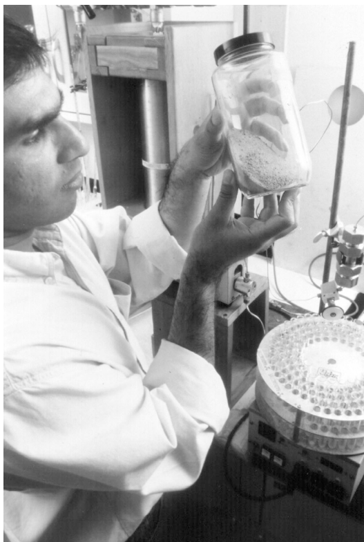
A column experiment to evaluate the kinetics and chemistry of surfactant flushing of hydrophobic organic contaminants from aquifer sediment. Courtesy of Richard Luthy, Carnegie Mellon University.
