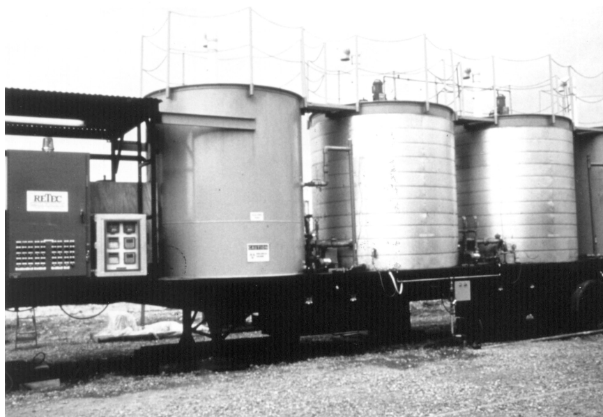
Large-scale complete mix pilot reactors are used to evaluate bioslurry treatment technologies. Courtesy of Remediation Technologies, Inc.
