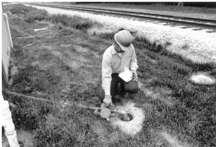
Sparging point being checked during regular site inspection. Courtesy of Fluor Daniel GTI.
