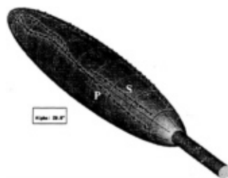
Figure 12. Comparison of constant current and constant temperature separation location topology on leeside for \alpha=20^\circ . Solid lines are steady constant current data. Dashed lines are steady constant temperature data. "P" indicates primary separation, while "S" indicates secondary separation.
