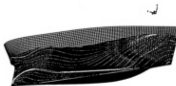
Figure 12, pressure and wall streamlines on the hull
