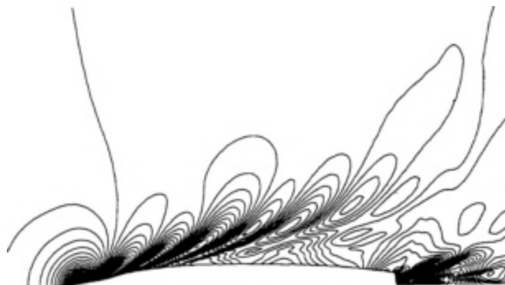
Figure 8: Free Surface Contours: 5415 Fr=0.2067
