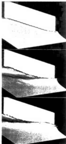
Figure 18: Perspective view of the computed bow waves about a 20° wedge model at three Froude numbers, Fd=0.8 , 1.1 and 1.4 from above.
