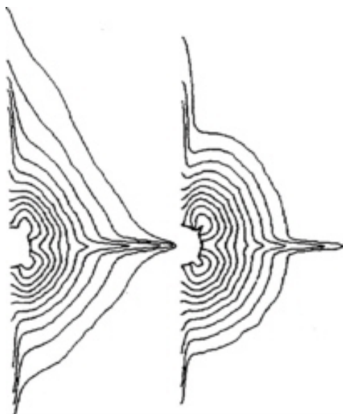
Figure 26 Taylor wake contours for RNG k- \epsilon turbulence model
