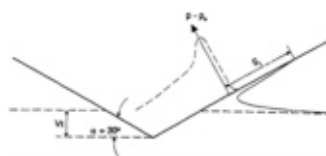
Figure 2: The free-surface elevation and pressure(p) distribution on the body surface during water entry of a symmetric wedge with constant velocity V. Deadrise angle \alpha=30^\circ . p_a is atmospheric pressure. The results are based on a similarity solution(Zhao and Faltinsen(1993)).
