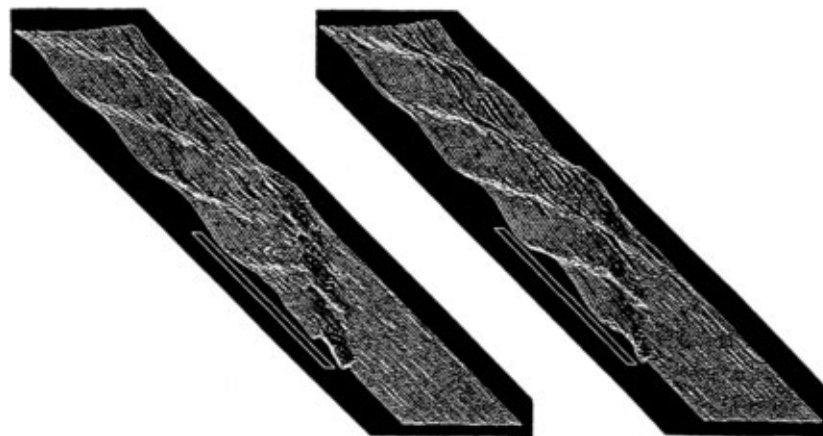
Figure 4: Diffraction Wave of a Series 60 ( C_B=0.8 ) at \omega t=0 , at Full Load ( left ) and Ballast ( right ) F_n=0.20 , \lambda/L=0.5
