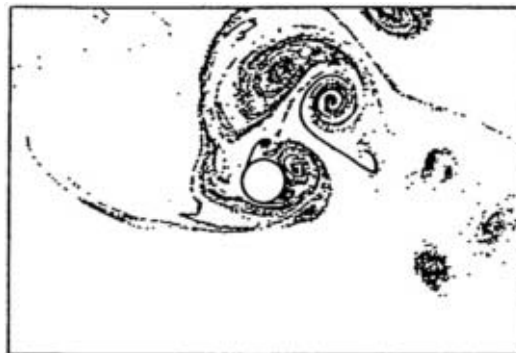
Figure 14 Numerical flow visualisation for KC=10 and \beta=70
