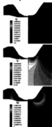
Figure 19 Computed (right) and measured (left) velocity field at x/l=+0.3 section
