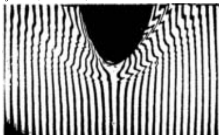
Fig. 3 Picture of free surface flow of NS12, Fn=0.15 , Rn=2.3 \cdot 10^5 .
