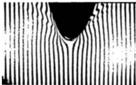
Fig. 3 Picture of free surface flow of NS12, Fn=0.15 , Rn=2.3 \cdot 10^5 .
