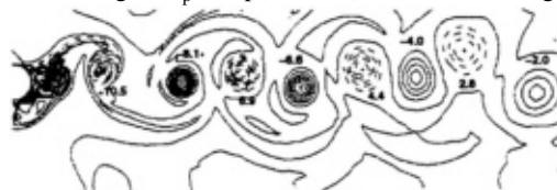
Figure 5: Typical Snapshot of the Vorticity in the Near Wake at Re=5600 .
