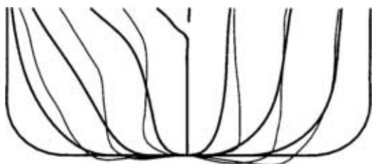
Fig. 7 Original and optimized hull, large range Thick lines—original hull Thin lines optimized hull
