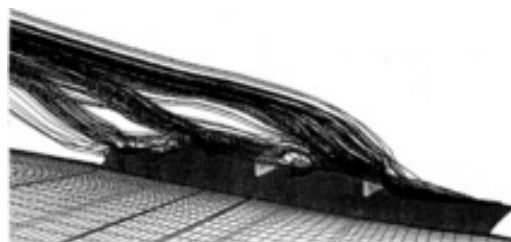
Fig. 8—Particle trace over DD-963 ship with 1-degree pitch and 5-degree roll at 15.44 m/s (30 knots) and wind angle of 30 degrees from starboard. Perspective view.
