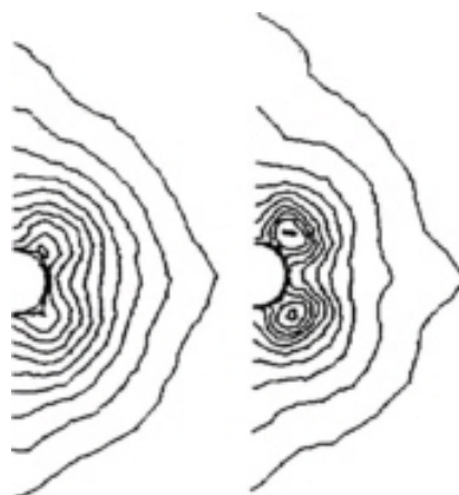
Figure 21 Taylor wake contours for unstructured grids
