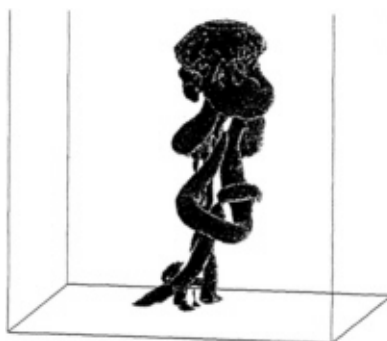
Figure 39: Iso-surface of the second-derivative of pressure in the flow-field about a rising bubble.
