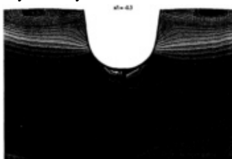
Figure 13, longitudinal velocity in x/l=-0.3 section for the coarse grid (left) and the fine grid (right)
