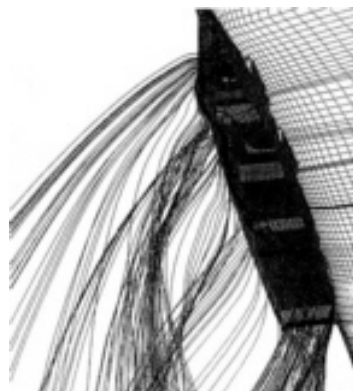
Fig. 7—Particle trace over DD-963 ship with 2-degree pitch at 15.44 m/s (30 knots) and wind angle of 30 degrees from starboard. Astern view.
