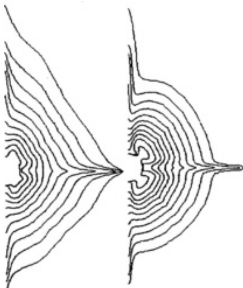
Figure 27 Taylor wake contours for Reynolds Stress model
