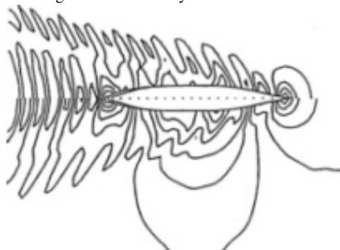
Fig. 5: Wave pattern for F_n=0.15 at h/T=3.2 (top) and h/T=1.5 (bottom)
