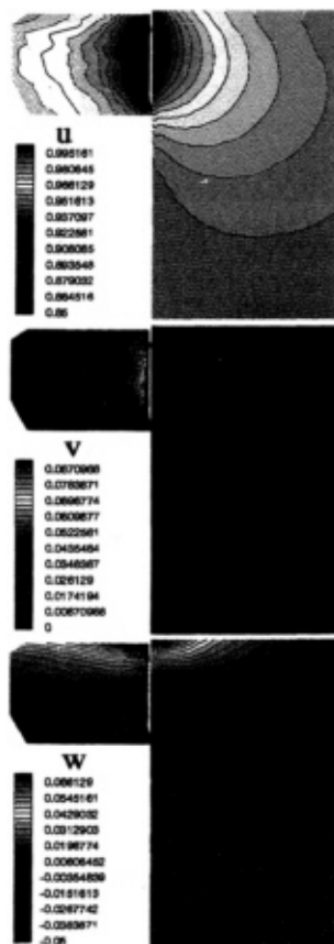
Figure 16 Computed (right) and measured (left) velocity field at x/l=-0.5 section
