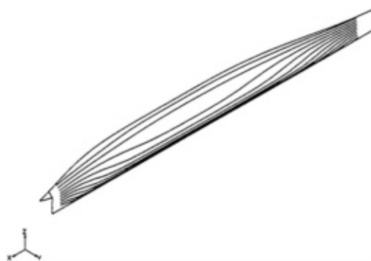
Fig. 5 Potential flow streamlines for boundary layer solution
