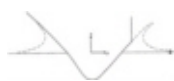
Figure 1: The (y,z) coordinate system, and the water entry of a body with flow separation on the right side and no separation on the left side.
