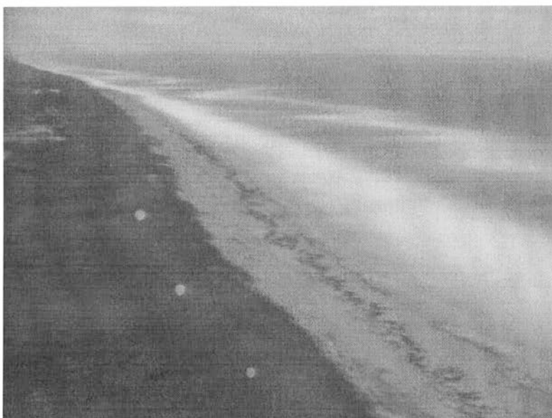
FIGURE 3-3 Black and white images taken by the ARGUS video monitoring system located near Duck, North Carolina. Position of breaking surf visible on short time exposure (a) is controlled by location of submerged bars. A ten-minute time exposure of the same section of beach (b) results in an image with useful information about the geometry and distribution of these offshore features. Photo courtesy of the Office of Naval Research.
