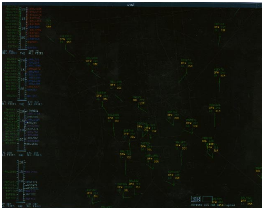
FIGURE 6.5 Center TRACON automation system (CTAS) final approach spacing tool (FAST) display. Source: National Aeronautics and Space Administration.
