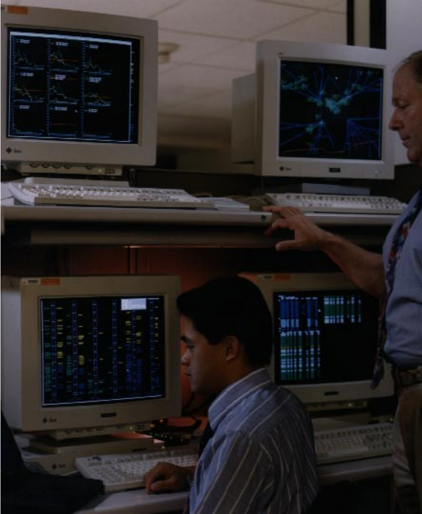
FIGURE 6.2 Center TRACON automation system (CTAS) traffic management advisor (TMA) display. Source: National Aeronautics and Space Administration.
