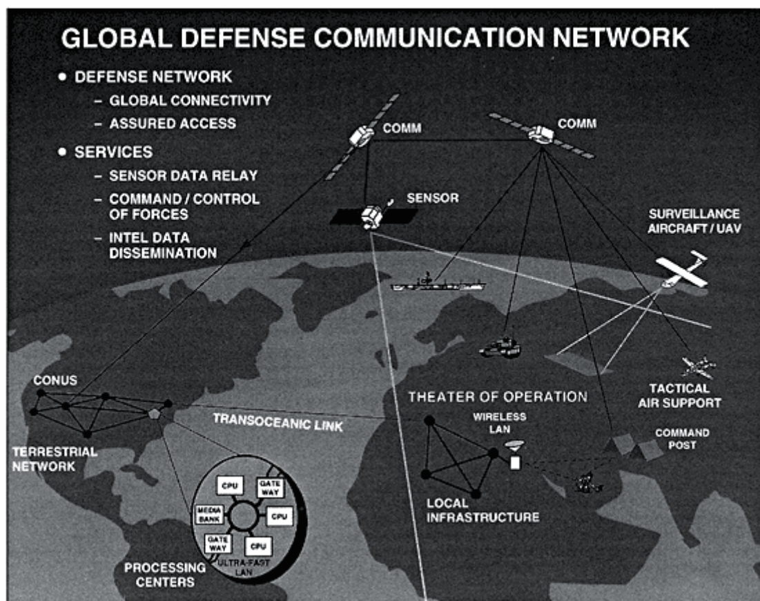
FIGURE 1.7 A schematic sketch of the global defense communication network. An essential element is the network in the sky consisting of interlinked communication satellites and sensor satellites. Extensive satellite networks are also planned for commercial mobile telephone and data service applications. The text discusses the capacity advantage of optical cross-links between the satellites of the network. (Courtesy of V Chan, MIT Lincoln Laboratory.)
