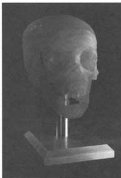
FIGURE 5.3 Skull model produced by three-dimensional rapid prototyping. (Courtesy of 3-D Systems, Inc.)
