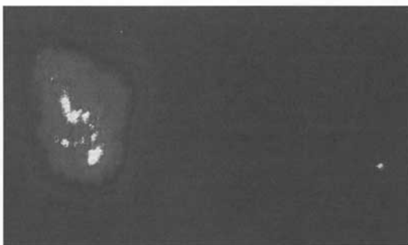
FIGURE 3.6 Telescope images with and without an atmospheric compensation adaptive optics system. The large, blurred patch at left is the star tau Cygni as seen without adaptive optics. The sharp, point-like image at right is the same star seen after correction by the atmospheric compensation system. (Courtesy of Mount Wilson Observatory.)
