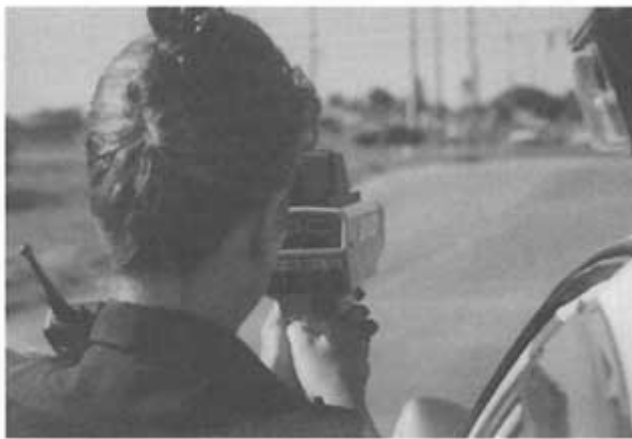
FIGURE 3.3 Laser radar used to measure traffic speed. The narrow laser beam can select one car from a group of vehicles, unlike conventional microwave radar. (Courtesy of the Institute of Police Technology and Management, University of North Florida.)
