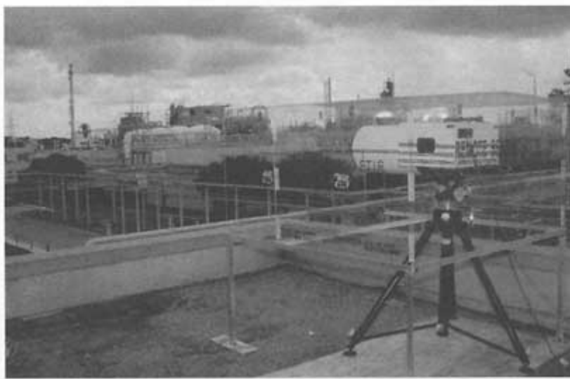
FIGURE 3.1 An optical-beam FTIR instrument used to measure gas emissions along the perimeter of an industrial chemical plant. (Courtesy of D.N. Hommrich, Essential Technologies, Inc.)
