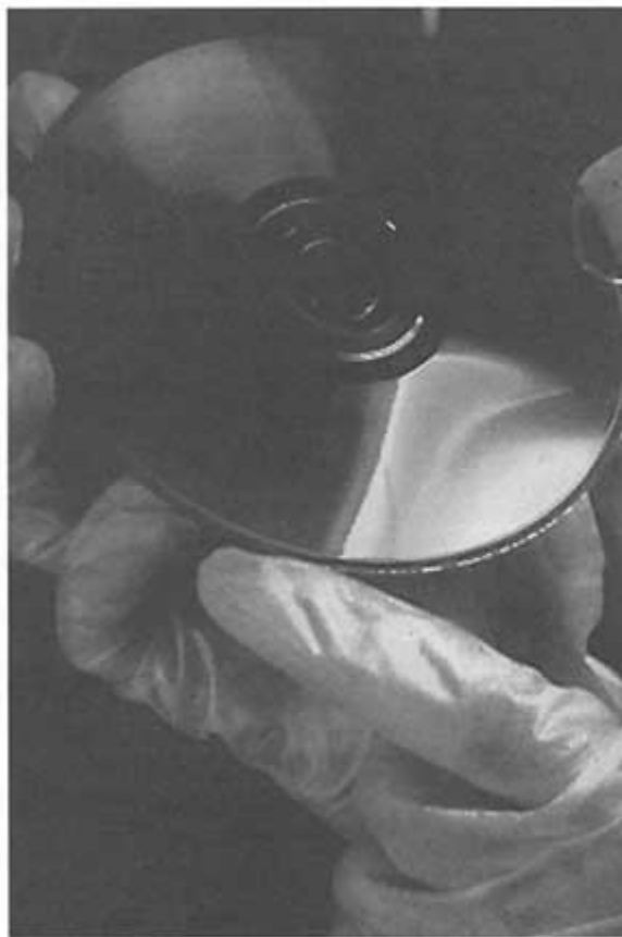
FIGURE 1.14 Compact optical disks. They may not be aware of it, but hundreds of millions of people have lasers in their homes. Lasers are hidden inside their compact disk players and computer CD-ROM (read-only memory) drives, which they use to read the information stored on compact disks such as the one shown here. These disks are made of injection-molded plastic. The information is stored digitally in the form of a pattern of pits pressed in the plastic. It is recovered by sensing changes in the reflection of a focused laser beam. Digital storage ensures high-quality reproduction of sound or data, and because the readout beam passes through the substrate, reproduction is insensitive to dust or scratches on the plastic surface. In addition, noncontact readout with a laser beam does not degrade the stored information in the way that passing a needle across a gramophone record did.
