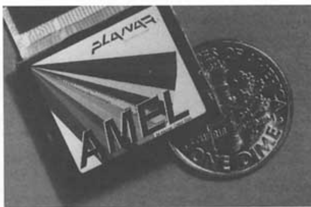
FIGURE 1.20 One future market expansion for displays is in flat, light, low-volume visual interfaces for personal digital assistants, Web browsers, augmented and virtual reality engines, and portable and wearable computers. The display shown here is a full-color VGA-sized device that carries nearly the information content of a personal computer monitor. (Courtesy of Planar America.)
