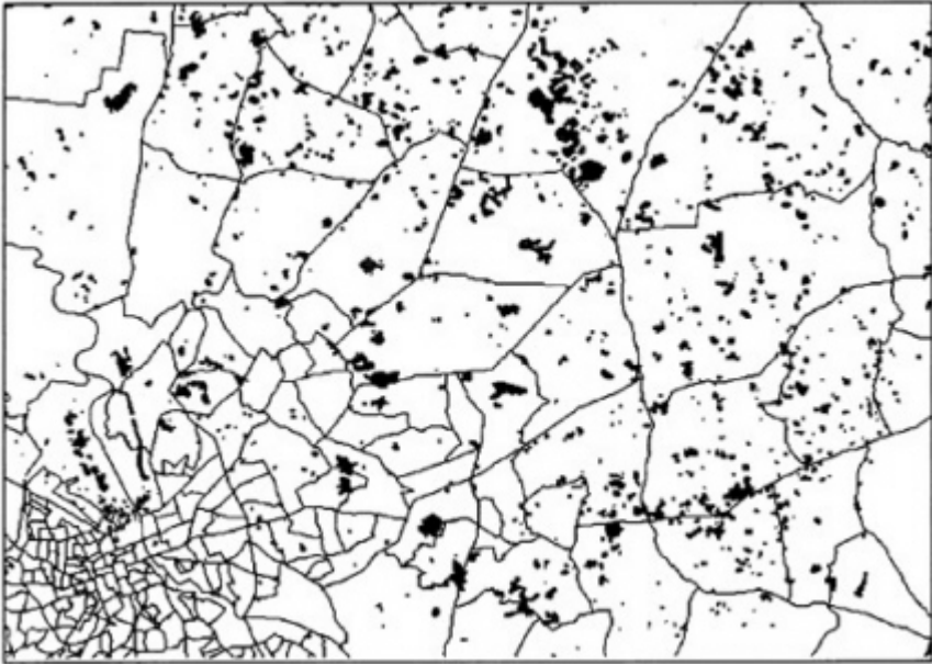
FIGURE 8-6 SPOT 10 × 10 m derived urban land-use changes within census block group polygons derived from SPOT 10 × 10 m data. 1990-1992 changes are in dark gray; 1992-1994 changes are in light gray.
