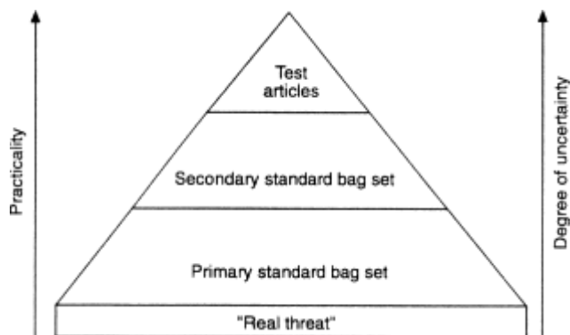
Figure 5-8 Schematic representation of the relationship between various levels of performance verification test objects and the "real threat" and the relative practicality and degree of uncertainty associated with them.
