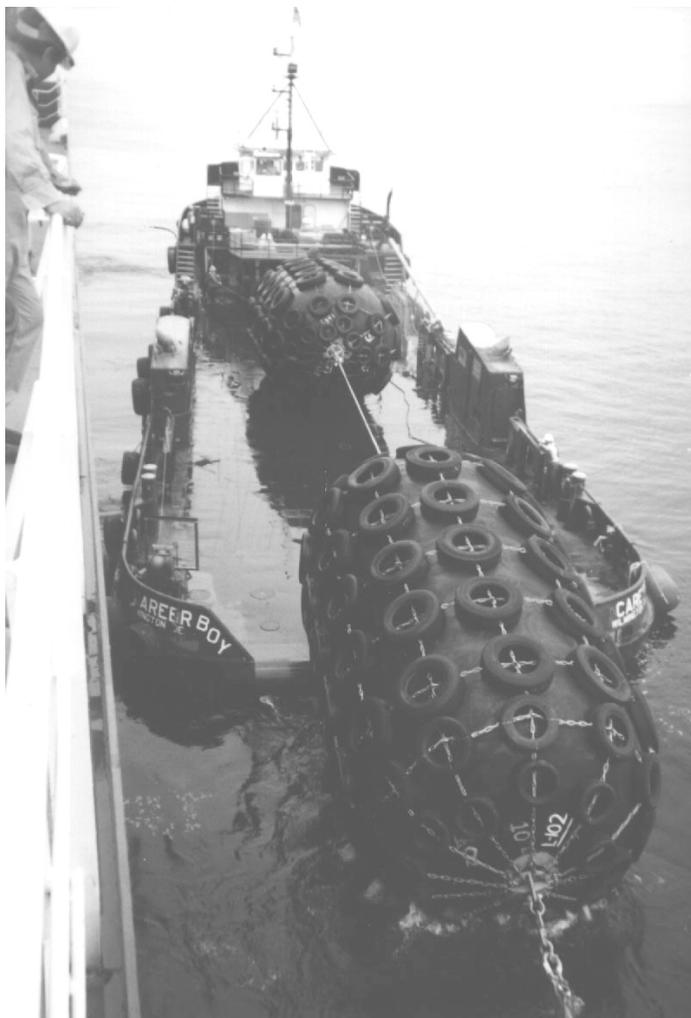
A workboat delivers fenders to a lightering operation. Photo Credit: Chevron Shipping Co.
