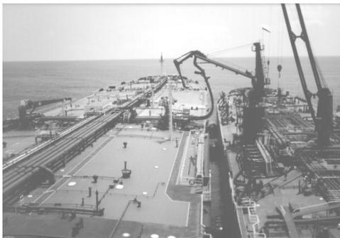
*In this case, the service vessel is equipped with a cargo crane to connect the transfer hoses. Photo Credit: Chevron Shipping Co.*
