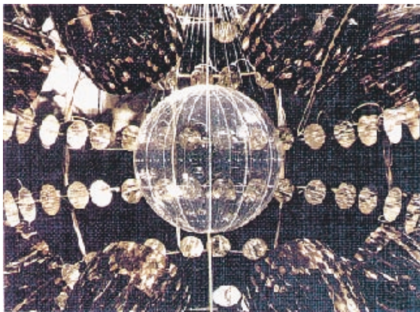
FIGURE 7.9 View of the prototype detector developed for the BOREXINO solar neutrino experiment at the Gran Sasso underground laboratory in Italy. The central 2-meter-diameter nylon sphere holds 4.5 tons of liquid scintillator and is surrounded by 1,000 tons of high-purity water. (Courtesy BOREXINO group.)
