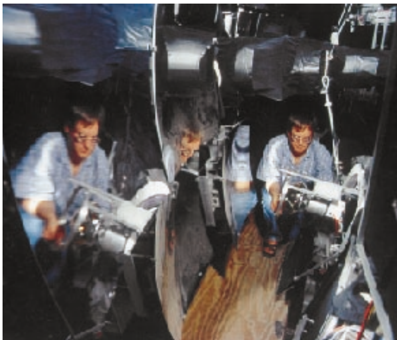
FIGURE 2.1.2 A part of the detector constructed at the University of Illinois, which is currently in use at the Bates accelerator to study small violations of mirror symmetry in electron-proton scattering. One of the collaborators is seen among the large reflectors used to focus radiation emitted by the scattered electrons. The experiment, initiated at the California Institute of Technology, is sensitive to the presence of the strangeness flavor in the quark-antiquark sea within a proton. (Courtesy of the MIT Bates Linear Accelerator Center.)
