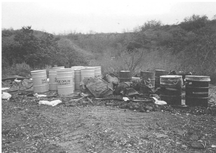
This collection of drums recovered during a time-critical removal action shows the diversity of tank condition. Courtesy of the U.S. Navy.
