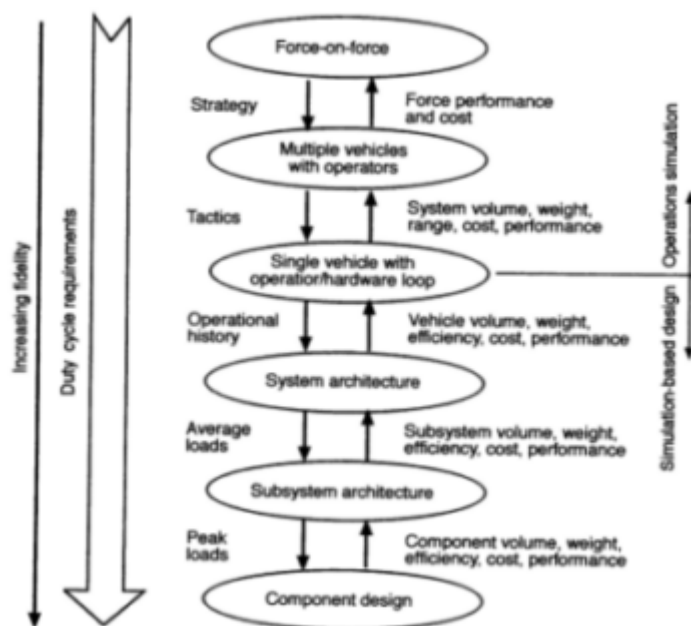
Figure 3-1 Hierarchical system of modeling and simulation for AAN trade-off analyses for a vehicle system.
