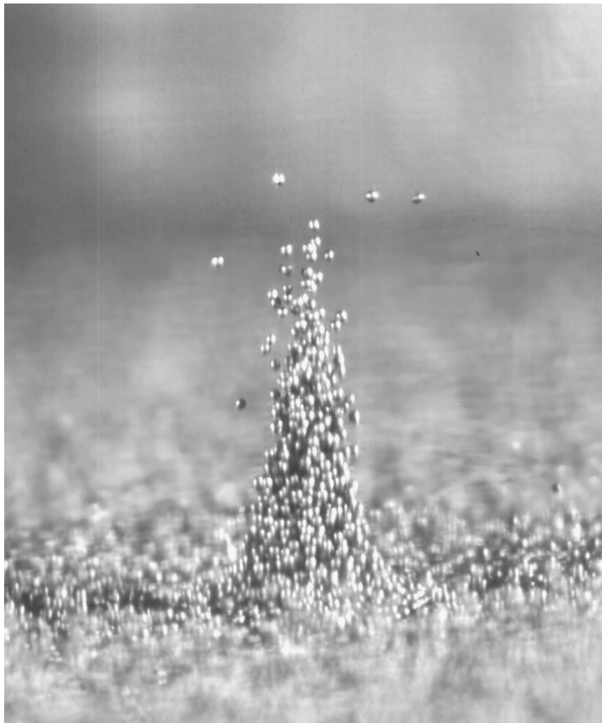
FIGURE 4.2 Localized standing wave in a vertically vibrated layer of 0.2 mm diameter bronze balls. (Courtesy of Center for Nonlinear Dynamics, University of Texas, Austin.)
