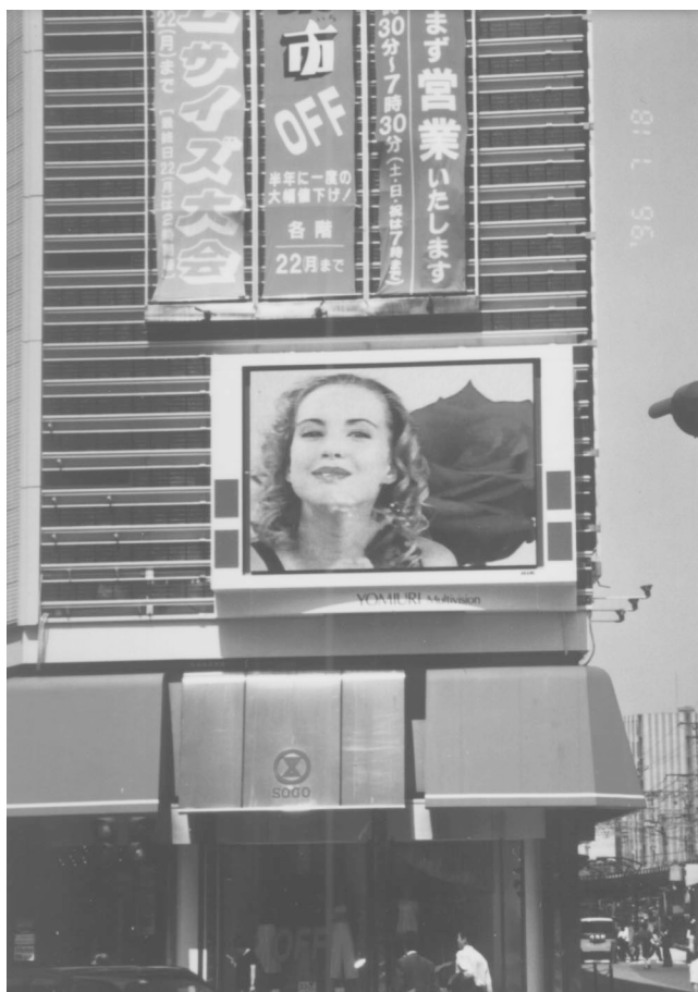
FIGURE 1.9.1 A black-and-white depiction of a full-color outdoor display incorporating blue and green InGaN LEDs and red GaAlAs LEDs. [ MRS Bulletin 22 , 30 (February 1997).]
