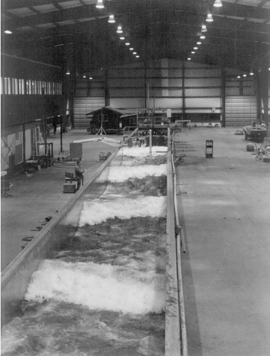
Large wave tank at the O.H. Hinsdale Wave Research Laboratory of Oregon State University (104.24 m long, 4.57 m deep, and 3.66 m wide). Used with permission from Charles K. Sollitt, Oregon State University.
