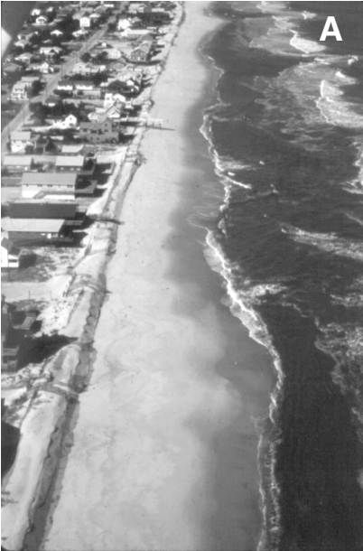
A. Fenwick Island, Delaware, in an eroded condition, with a short beach offering little storm protection or recreational function.
