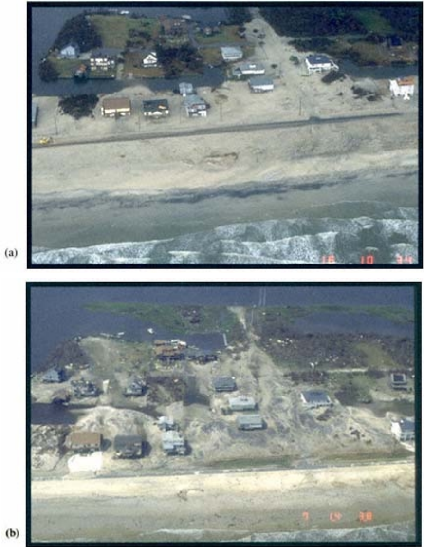
PLATE 6 West Onslow Beach, N.C. overflow ( 34^{\circ} 30.70'N , 77^{\circ} 22.16'W ). (a) After Hurricane Bertha, 7/16/96, 10:34 EDT. (b) After Hurricane Fran, 9/7/96, 14:38 EDT. Areas overwashed by Hurricane Bertha were more susceptible to erosion and overwash by Hurricane Fran. Initially susceptible to erosion during a category 2 hurricane, the area affected by the category 3 storm was greatly expanded. (Stumpf et al., 1996).
