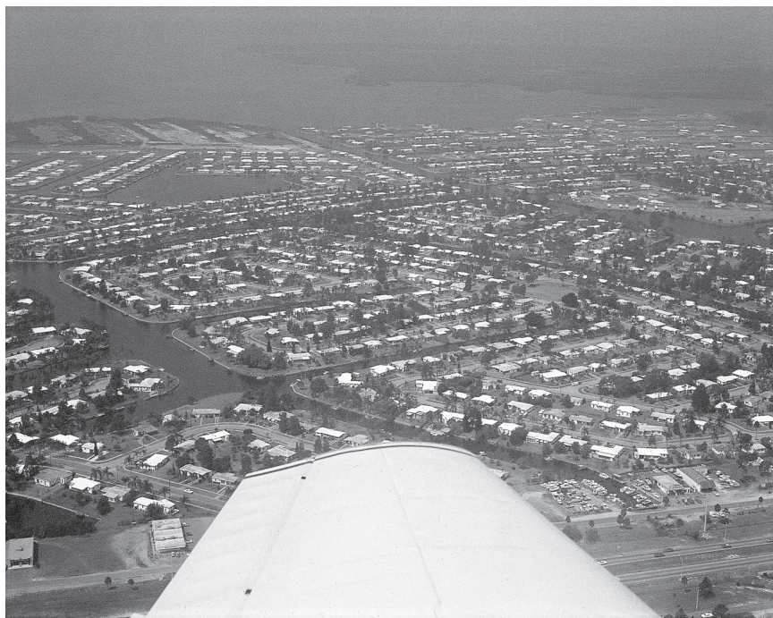
FIGURE 9-4 Finger canals in the Port Charlotte, Florida area, in 1974. Systems of canals with dead-ends have reduced circulation and flushing and can lead to accumulation of pollutants and nutrients, with resultant eutrophication problems (photo by W. Huber).
