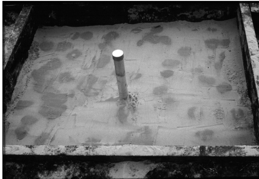
FIGURE 5-8 Unstable wetting patterns at 0.20 m depth in wettable sand after 403 mm precipitation; dark spots are wet. From Hendrickx and Dekker (1991).
