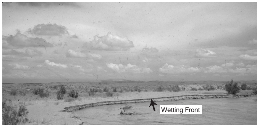
FIGURE 5-5 Stable wetting front in a loam soil along the Rio Salado near Socorro observed in August, 1995, after a few days with heavy rainfall. The wetting was exposed after the river bank collapsed shortly before the picture was taken by Hendrickx..
