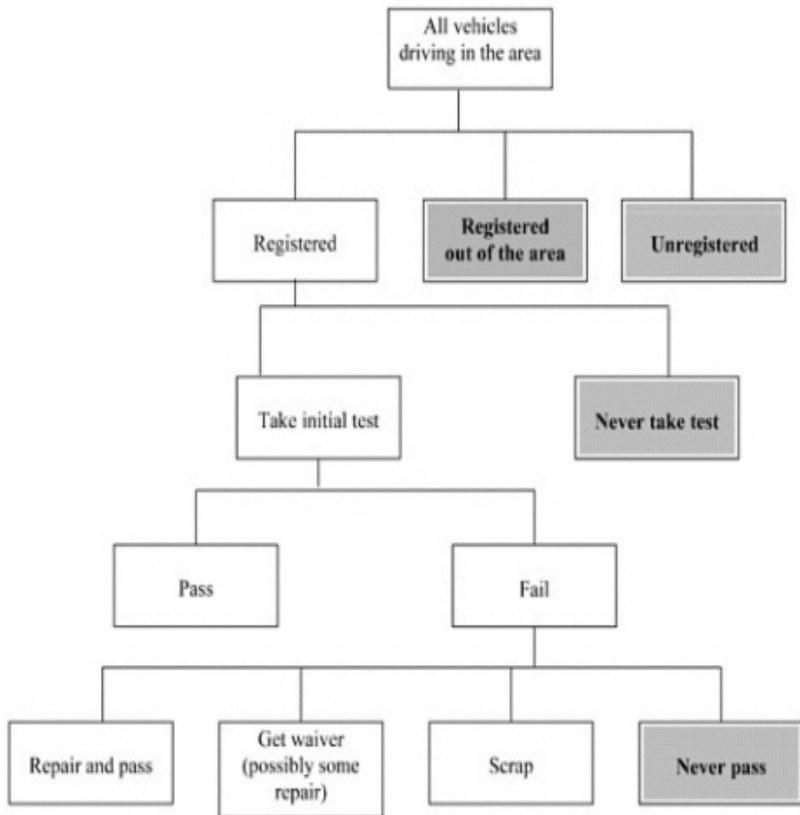
FIGURE 5–2 Classification of vehicles in an area subject to I/M. Shaded boxes indicate noncomplying vehicles. Source: Adapted from Harrington et al. 1998.
