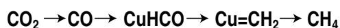
FIGURE 5.7 Sequence of the electrochemical reduction of CO 2 with copper to form methane.
