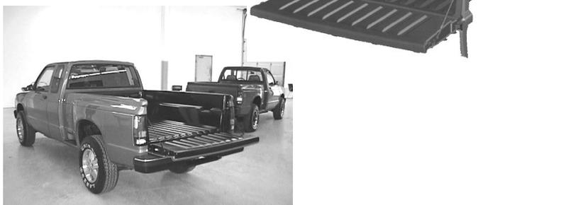
FIGURE 2-2 Polymer composite pickup box.
