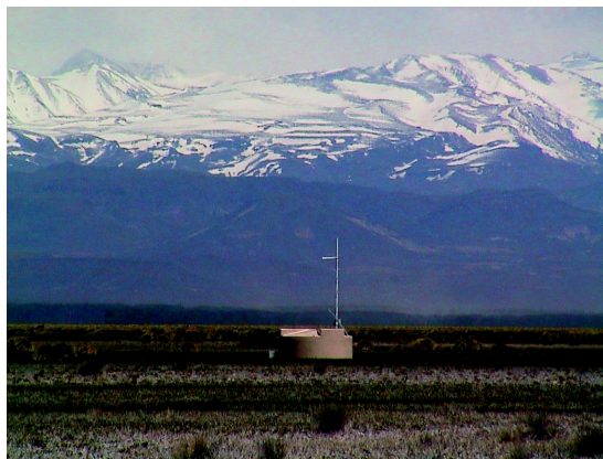
FIGURE 6.1.1 (a) Illustration of a ground-based array of Cerenkov water detectors for detecting shower particles with a fluorescence detector for imaging the atmospheric cascade generated by ultra-high-energy cosmic rays. (b) An array of phototubes suspended in ice that senses interactions of upward-going neutrinos; it uses the bulk of the Earth to filter out other types of particles; adapted from image courtesy of the IceCube Collaboration. (c) One of the Cerenkov shower detectors in the Pierre Auger Observatory array in Argentina; image courtesy of the Pierre Auger Observatory.
