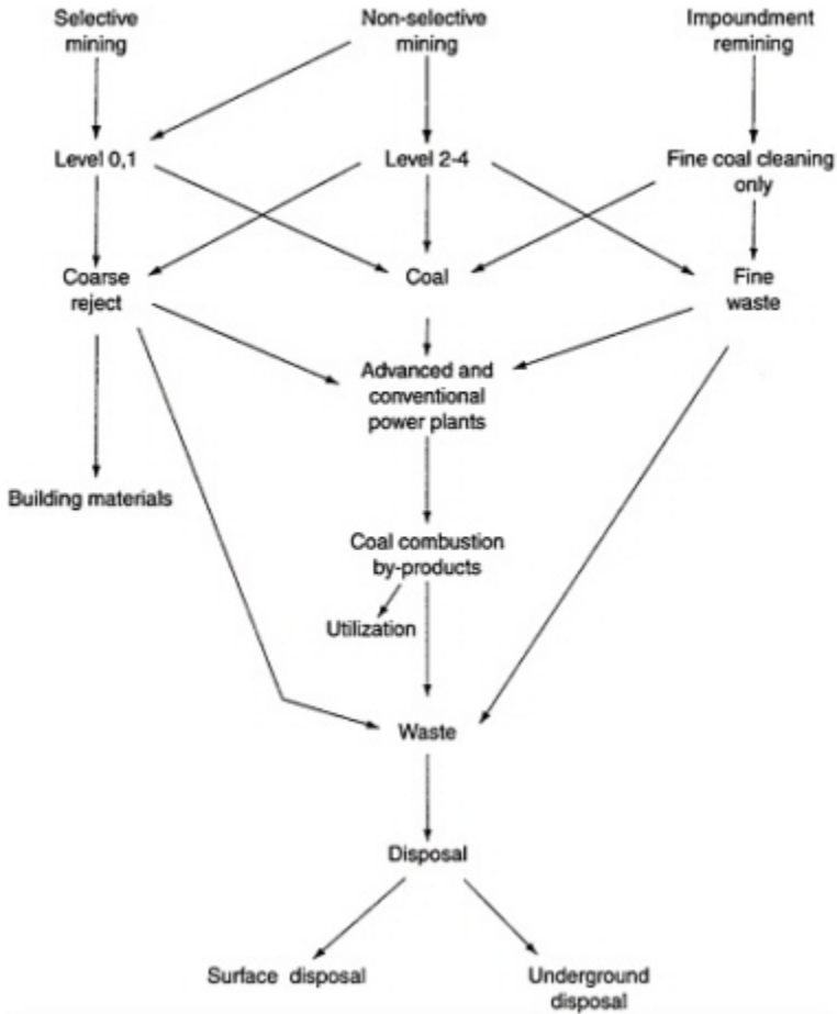
FIGURE 7.1 Coal system: Mining, preparation, utilization, residues, and disposal.
