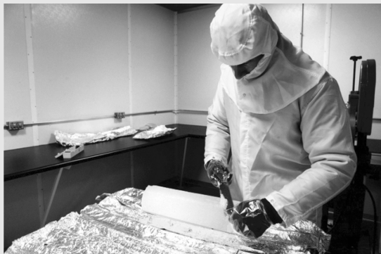
Scientist cleaning a piece of ice core in the cold clean room. SOURCE: Geoffrey Hargreaves, NICL.
