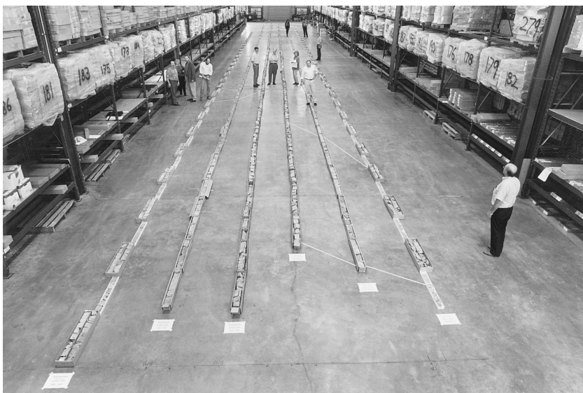
FIGURE 2-1 1,000 feet (333 boxes) of rock core laid out inside the Bureau of Economic Geology Core Facility, University of Texas at Austin. These rows represent data from four wells. Given the average increase in core and cuttings holdings annually, these 333 boxes represent approximately 2 months of average growth (see discussion in Sidebar 3-4). SOURCE: David M. Stephens, Bureau of Economic Geology, The University of Texas at Austin.
