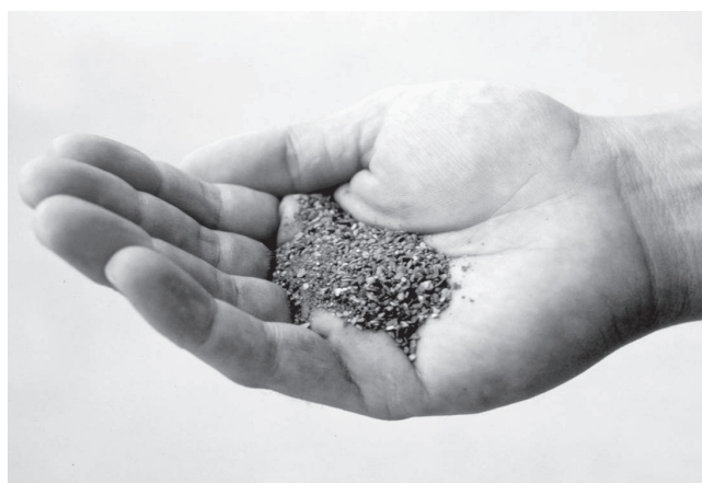
FIGURE 3-3b Cuttings. SOURCE: Baker, 1980. Petroleum Extension Service, The University of Texas at Austin.
