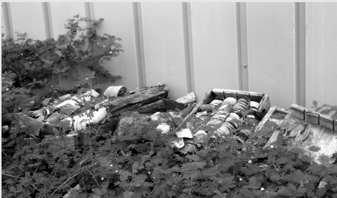
Cores stored outside at Oakridge National Laboratory, Tennessee, in Spring 2001. These cores are from the Tennessee Valley Authority's Clinch River Breeder Reactor site. Rescue of cores in this state of degradation is unlikely given the probable loss of documentation associated with them. SOURCE: Richard Pawlowicz, Bechtel National, Inc., San Diego, California.
