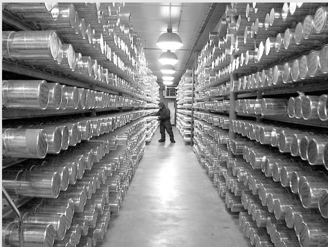
Inside the National Ice Core Laboratory. The ice core storage room is maintained at a temperature of -33^{\circ}\text{F} ( -36^{\circ}\text{C} ). About three-quarters of the NICL collection is in 1-meter (3.3-foot) tubes, the other quarter is in 1.5-meter (5-foot) tubes. Each tube contains part of a single core. SOURCE: Geoffrey Hargreaves, NICL.
