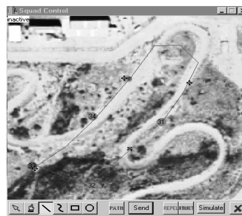
FIGURE 4-5 User interface for perimeter surveillance. The perimeter is marked in blue and miniature intrusion detection sensors are marked by circular numbered icons. An alarm is identified when the icon turns red. The vehicles closest to the intrusion attend to the alarm, while the others adjust their position around the perimeter to prepare for other possible alarms. SOURCE: Feddema et al. (2002). © 2002 IEEE.
