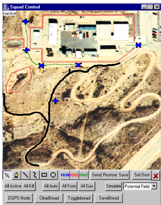
FIGURE 4-6 User interface for a facility reconnaissance mission. The initial positions of the vehicles were at the lower left corner of the screen. The vehicles first follow their assigned paths (drawn in black). Once they reach the end of their paths, the vehicles use a potential field path planner to avoid obstacles (drawn in red) and navigate towards goal attractors (drawn in green). To avoid collision between the vehicles and to uniformly cover the goal attractors, repulsive forces push the vehicles away from each other. The path plan is first previewed by the operator, after which the goal and obstacle polygons are downloaded to the vehicle and the same potential field path planner drives the vehicles toward the goal polygons while avoiding obstacle polygons, unplanned obstacles, and neighboring vehicles. The final path is not necessarily the same as the previewed paths since the potential field path planner will avoid sensed obstacles that were not in the original map and the real position of neighboring vehicles may be different at the time of execution. SOURCE: Feddema et al. (2002). © 2002 IEEE.
