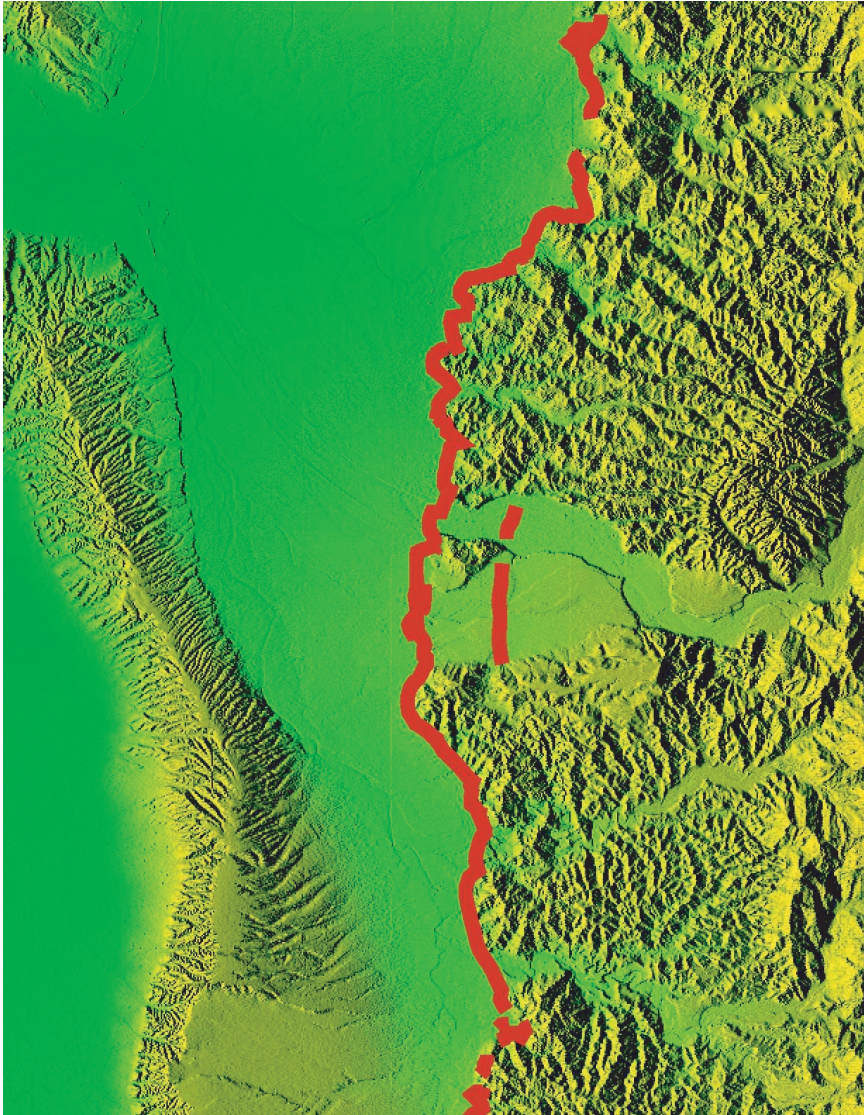
FIGURE 4.22 Shaded-relief map made from a 40-meter digital elevation model of Taiwan, used in mapping active faults and folds. Geomorphic expression of the Chelungpu fault (red line), the cause of the M 7.6 Chi-Chi earthquake in 1999, is clearly expressed. SOURCE: Charles Rubin, Central Washington University, Ellensburg, and Kerry Sieh, Caltech.
