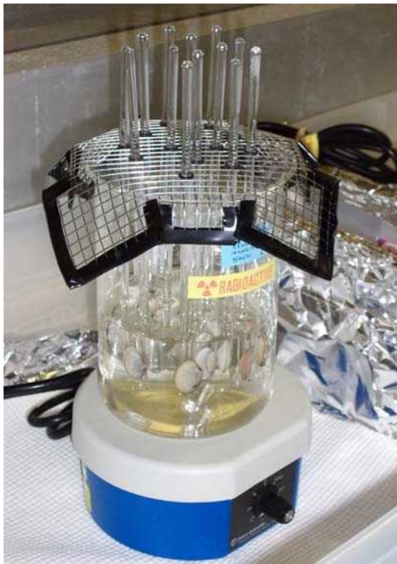
Laboratory set-up for measuring assimilation efficiency of clams.
