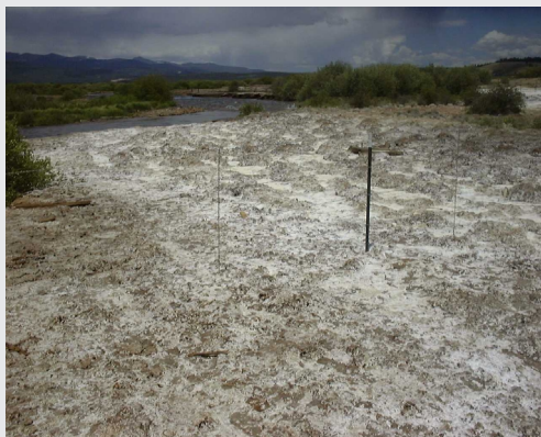
Alluvial tailings deposits along the Upper Arkansas River outside Leadville. Surface salt consists of metal sulfates with zinc concentrations as high as 9 percent.
