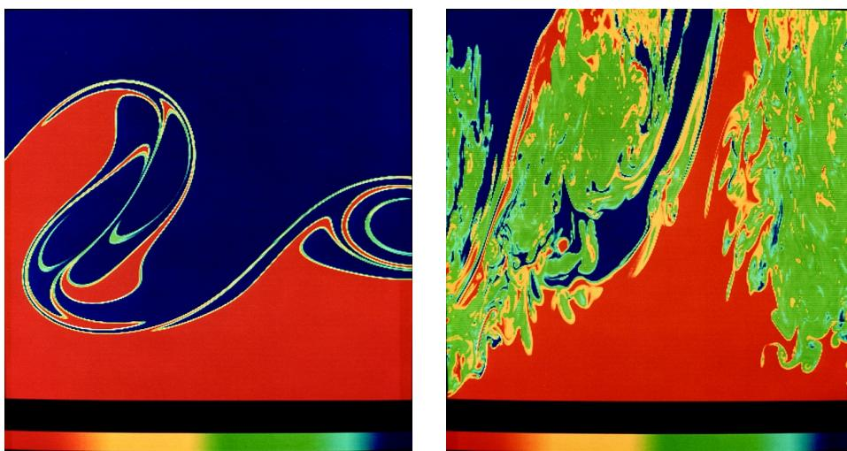
FIGURE 3.5 Shear-layer scalar field. Blue: pure high-speed fluid. Red: pure low-speed fluid. Color bars denote intermediate compositions. Left:  $Re = 2.3 \times 10^3$ ; right:  $Re = 2.0 \times 10^4$ . Courtesy of P. Dimotakis, California Institute of Technology and M.M. Koochesfahani, Michigan State University.
