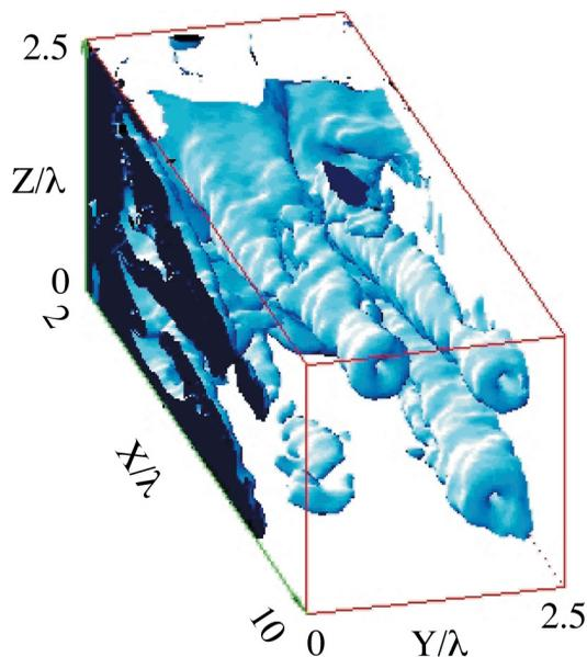
FIGURE 4.4 Three-dimensional particle-in-cell simulations of energetic electron generation and transport with laser pulses in overdense plasmas. Contours of magnetic-field structure due to the Weibel instability are shown. Courtesy of Y. Sentoku, General Atomics.
