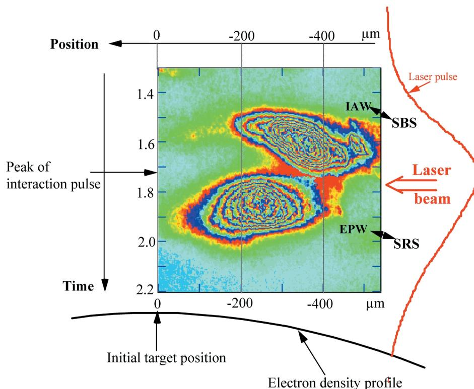
FIGURE 4.10 Measurements in space and time of the amplitudes of both electron plasma and ion sound waves in a laser-irradiated plasma. SOURCE: Reprinted, with permission, from C. Labaune, H.A. Baldis, N. Renard, E. Schifano, and A. Michard, 1997, "Interplay Between Ion Acoustic Waves and Electron Plasma Waves Associated with Stimulated Brillouin and Raman Scattering," *Phys. Plasmas*, 4:423-427, copyright 1997 by the American Institute of Physics.
