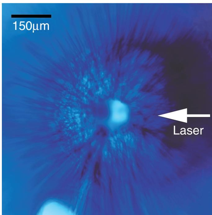
FIGURE 4.7 Image of a laser-heated 150-micron balloon target using proton radiography. The target was heated by a laser; the fine structures shown in the image are due to plasma electric fields that deflect the protons. Courtesy of M. Borghesi, Queen's University, Belfast; O. Willi, A. Schiavi, M. Haines, and H. Campbell, Imperial College, London; S. Hawkes and R.C. Clarke, Rutherford Appleton Laboratory; and A.J. Mackinnon, Lawrence Livermore National Laboratory.
