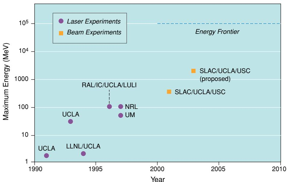
FIGURE 4.2 Progress in plasma accelerator energy: maximum energy gains and laboratories where they were obtained.
