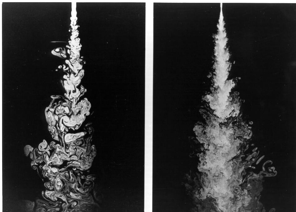
FIGURE 3.6 Jet-fluid concentration field in the plane of symmetry of turbulent jets. Left:  $Re = 2.3 \times 10^3$ ; right:  $Re = 10.0 \times 10^3$ . Courtesy of P. Dimotakis, California Institute of Technology.
