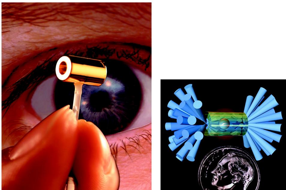
FIGURE 4.3 Images of the type of hohlraum used for ignition experiments. The schematic on the right shows the hohlraum irradiated by 192 NIF beams. Courtesy of Lawrence Livermore National Laboratory.
