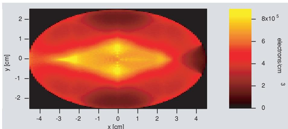
FIGURE 4.9 Simulated time-averaged electron-cloud density in a field-free region in the arcs of the PEP-II positron ring. The beam (not shown) occupies a small region at the center of the chamber, of order 1 mm in diameter. Courtesy of M.A. Furman, Lawrence Berkeley National Laboratory.
