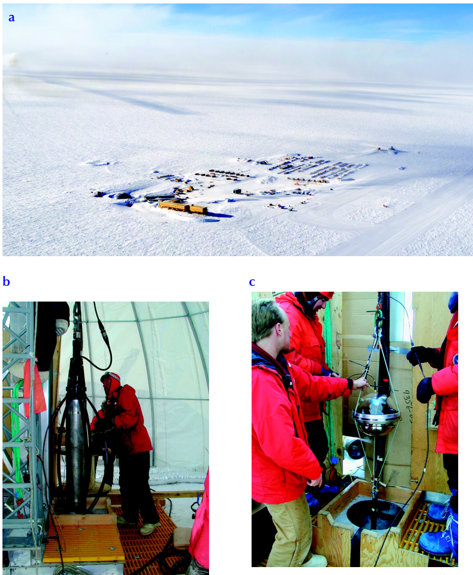
FIGURE 3.2 (a) An aerial view of the Amundsen-Scott South Pole research station, where IceCube will be located. The station sits on a 2,700-m thick plateau of snow-covered ice. Image courtesy of USAF MSgt. David McCarthy and the National Science Foundation. (b) Teams of scientists and engineers use a hot-water drill to bore holes deep into the ice. Strings of light sensors are deployed in the holes. (c) Lowering one of the strings of light sensors; the glass capsule encases the photomultiplier tube. Once the water in the bore-hole refreezes, it will be impossible to access the sensors. Images courtesy of the AMANDA Collaboration, the IceCube Collaboration, and the National Science Foundation.
