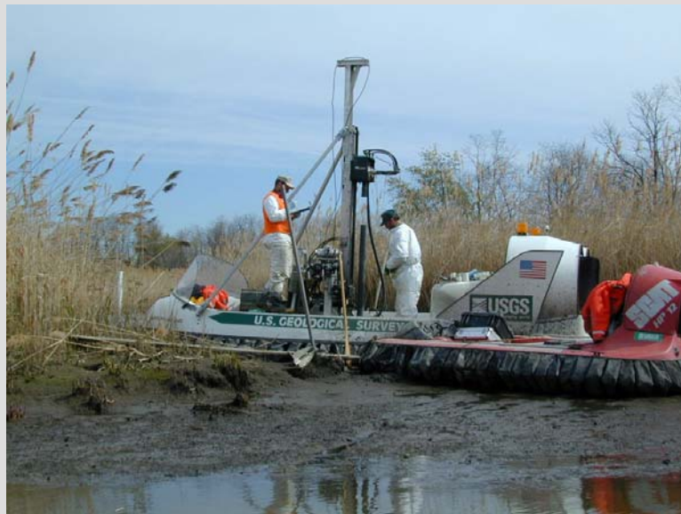
The Hoverprobe and a support hovercraft during drilling and water-quality profiling along the West Branch, Canal Creek, Aberdeen Proving Ground, MD. The support hovercraft was used for transport of samples to nearby laboratory facility for immediate analysis and in case emergency exit was needed.
