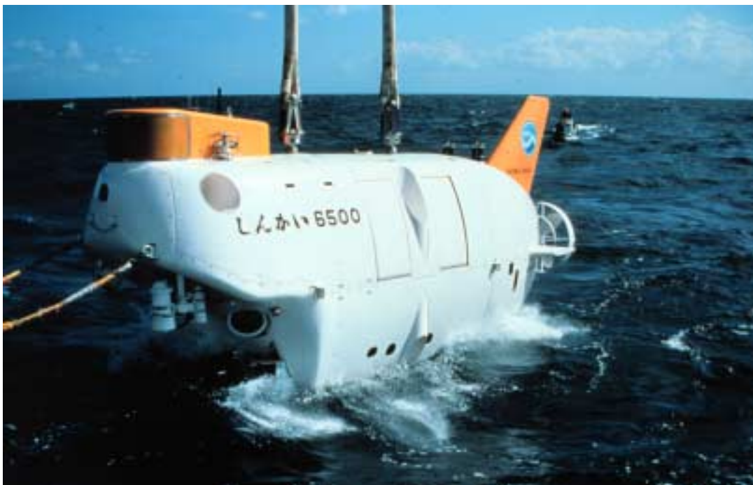
Figure 7. SHINKAI 6500 is rated to 6500 meters, deepest active sub in the world.
