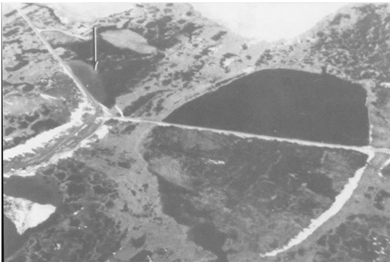
FIGURE 7-2 One of the four lake basins along the Waterflood road at Prudhoe Bay. The photo was taken in early summer before ice in the culverts thawed. By late summer the large oval impoundment drained, but the vegetation changed over a period of 3 years. Notice the lack of elevated microsites for bird nests in the flooded areas compared with the other side of the road. Also note the other impoundment along the road (arrow), which does not drain all summer. SOURCE: Walker 1996. Reprinted with permission, copyright 1996, Springer-Verlag.
