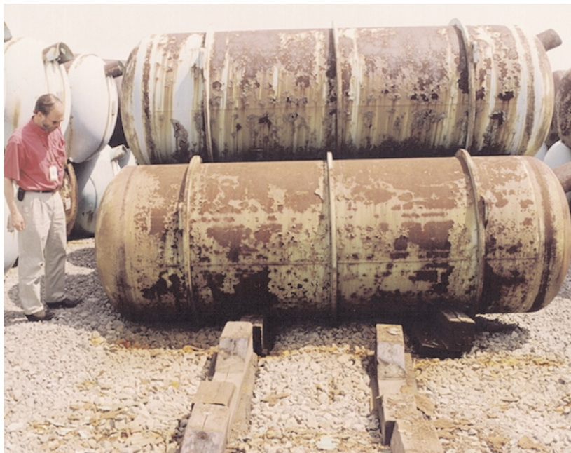
Figure 6.1 Cylinders containing about 14 tons of depleted-uranium hexafluoride are stored outdoors. These cylinders are made of carbon steel with wall thickness of 1/4 or 5/16 inch. The stacking arrangement often prevents worker access for inspection or maintenance. Source: http://web.ead.anl.gov/uranium/guide/ .
