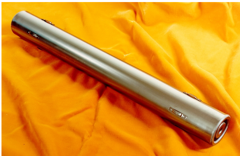
Figure 4.1 Fuel from the Hanford N-Reactor comprises 85 percent of DOE's spent nuclear fuel inventory. The fuel consists of metallic uranium assemblies (two concentric cylinders with zirconium-based cladding) that are 66 cm long and 5 cm in diameter. In fresh fuel, as shown here, the U-235 enrichment is 1.25 percent. Source: DOE Richland.
