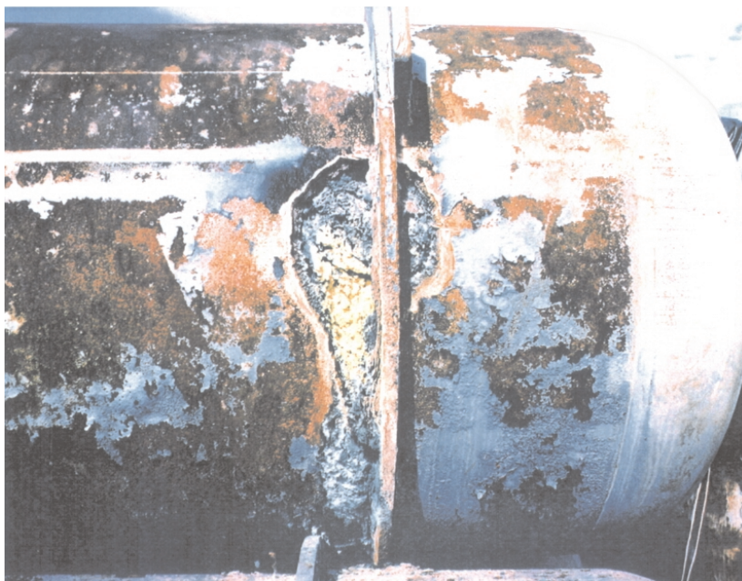
Figure 6.3 Corrosion has breached the walls of some cylinders. Breaches have tended to be self-sealing. They are repaired by welding a patch over the opening.
