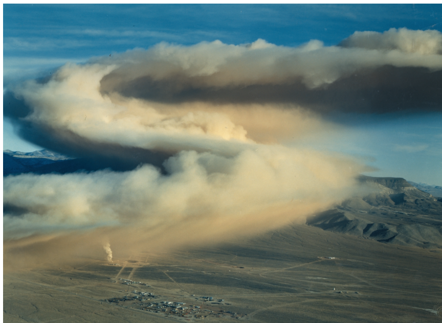
FIGURE F.2 Photograph of plume from underground Shot BANE BERRY showing separation of lower and upper portions due to different directions of winds near the ground and aloft.
