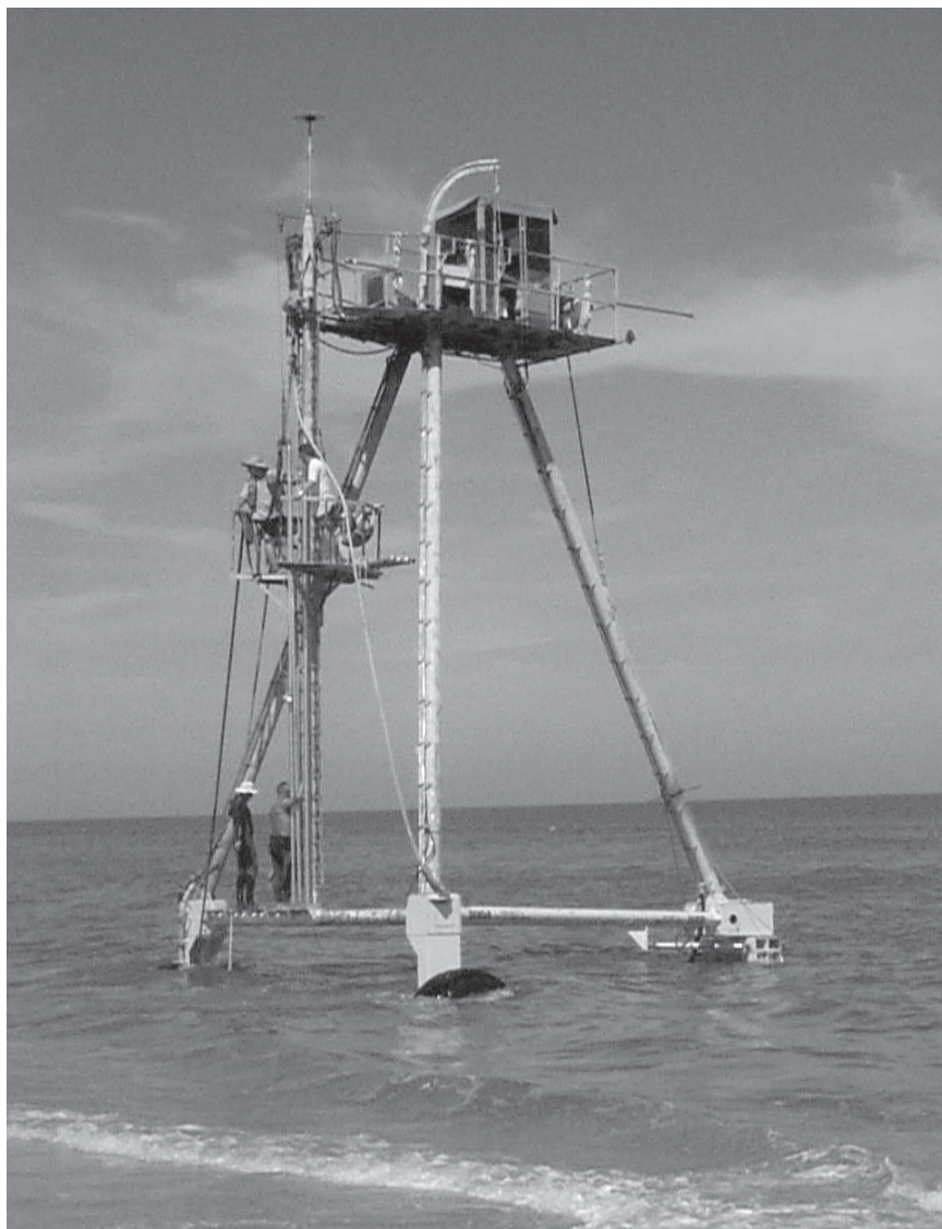
FIGURE 2-3 The USACE FRF's Coastal Research Amphibious Buggy ( CRAB ). This deployment and retrieval platform is a tower on three wheels, hydraulically driven by a diesel engine located on the operations platform, 11 m above the seabed. The CRAB can operate in 2 m high breaking waves in 10 m depth of water, with Global Positioning System (GPS)-positioning accuracy to deploy fluid- and sediment-boundary layer sensors. The CRAB has also been used to measure monthly bathymetric changes at the Duck, NC site over the past 25 years. Figure courtesy of Joan Oltman-Shay, NorthWest Research Associates, Inc.
