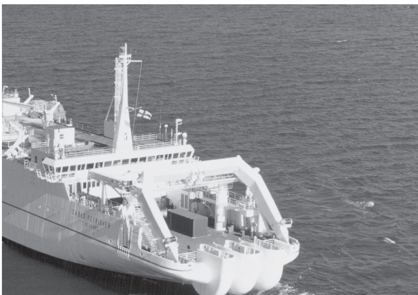
FIGURE 5-2 Photo of the Cable Retriever , a state-of-the-art, purpose-designed, all-stern working cable ship, equipped with an ROV (full view top; rear view bottom). This 117 m long vessel has a storage capacity of some 2,475 tons of cable. Specialized vessels such as this will be required for observatory cable installation and repair. Figure courtesy of Global Marine Systems Limited.
