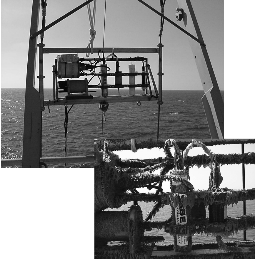
FIGURE 2-1 This before-and-after picture shows the tremendous problem that biofouling presents to the long-term deployment of instruments in the upper ocean, especially in coastal regions. Figure courtesy of Richard Jahnke, Skidaway Institute of Oceanography.
