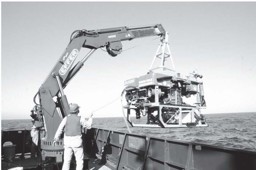
FIGURE 5-3 ROVs like the Jason II (above), will be the work-horses of ocean observatories. ROVs will be needed for installation of seafloor observatories, connecting moorings to seafloor junction boxes, installing experiments, and servicing or repairing instruments and network equipment on the seafloor. Jason II was designed for detailed survey and sampling tasks that require a high degree of maneuverability. Jason II is operated by the U.S. National Deep Submergence Laboratory at WHOI. Figure courtesy of ©Woods Hole Oceanographic Institution.
