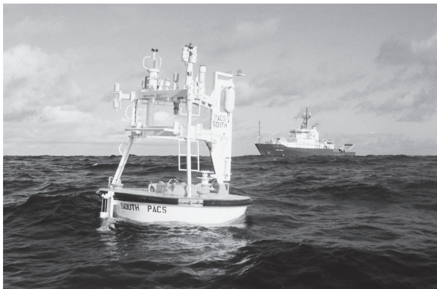
FIGURE 4-5 Surface moorings such as this one will need to be serviced annually, requiring up to one month of ship time (including transits) for each of the widely spaced moorings of the OOI global observatory network. Figure courtesy of Woods Hole Oceanographic Institution.
