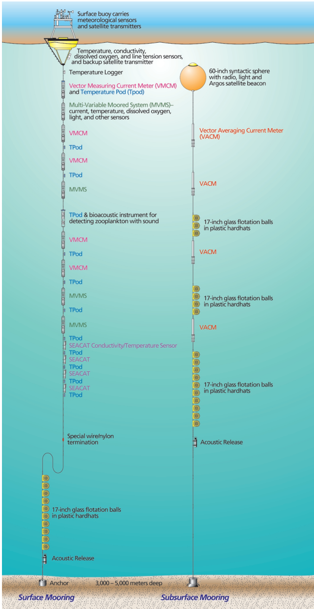
PLATE 4 Conventional surface (left) and sub-surface (right) moorings currently operational at many tropical and mid-latitude sites designed to measure meteorological, air-sea, and upper-ocean properties. Figure courtesy of Jayne Doucette, ©Woods Hole Oceanographic Institution.
