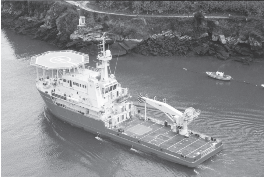
FIGURE 5-1 Photo of the Midnight Arrow , an offshore energy industry Class 2 sub-sea construction vessel. Vessels like this with a heavy lift capacity, large load capacity, and ample deck space would be ideally suited for deploying large spar buoys and moorings and seafloor node installation, maintenance, and replacement. Figure courtesy of Torch Offshore, Inc.
