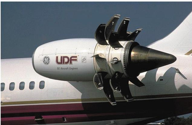
FIGURE 4-2 Unducted fan demonstrator ready for flight. Source: Burkhard Domke, Grünendeich, Germany. Available online at <[www.b-domke.de/AviationImages/Rarebird/0809.html](http://www.b-domke.de/AviationImages/Rarebird/0809.html)>.
