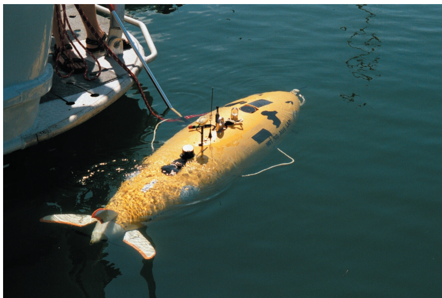
FIGURE 6.3 Autonomous underwater vehicles use programmed routes and sampling protocols to collect oceanographic data. (A) Xanthos , designed at the Massachusetts Institute of Technology, can dive to 3,000 m (used with permission from the Massachusetts Institute of Technology Sea Grant). (B) The Autonomous Benthic Explorer (ABE) can dive to 5,000 m. It is 2 m long and can cruise at 2 knots. On-board equipment includes a conductivity, temperature, and depth device; sonar; video cameras; and a magnetometer (used with permission from the Woods Hole Oceanographic Institution).
