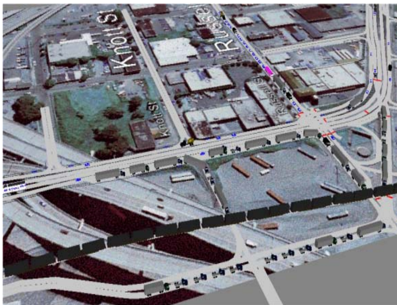
FIGURE 7 Revised traffic simulation model at midday with Train 100 event. UPRR train blocks the Russell and Knott Street accesses, resulting in truck queuing on Interstate Avenue.
