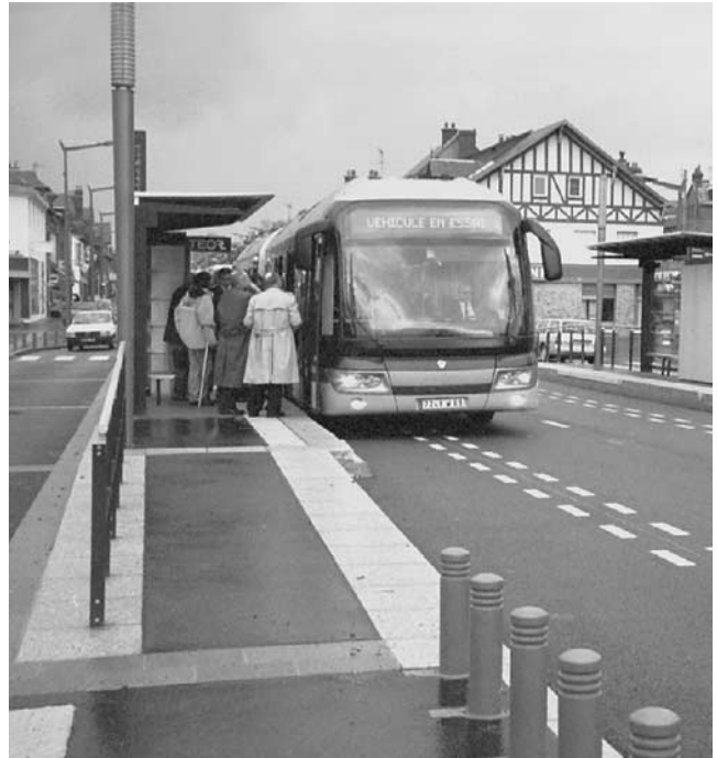
Photo 7-I. "Optical scanner" vehicle at station.
