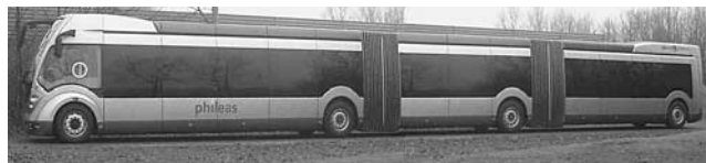
Photo 6-Y. 24-meter (80-foot) hybrid, magnetically guided, modular BRT vehicle.
