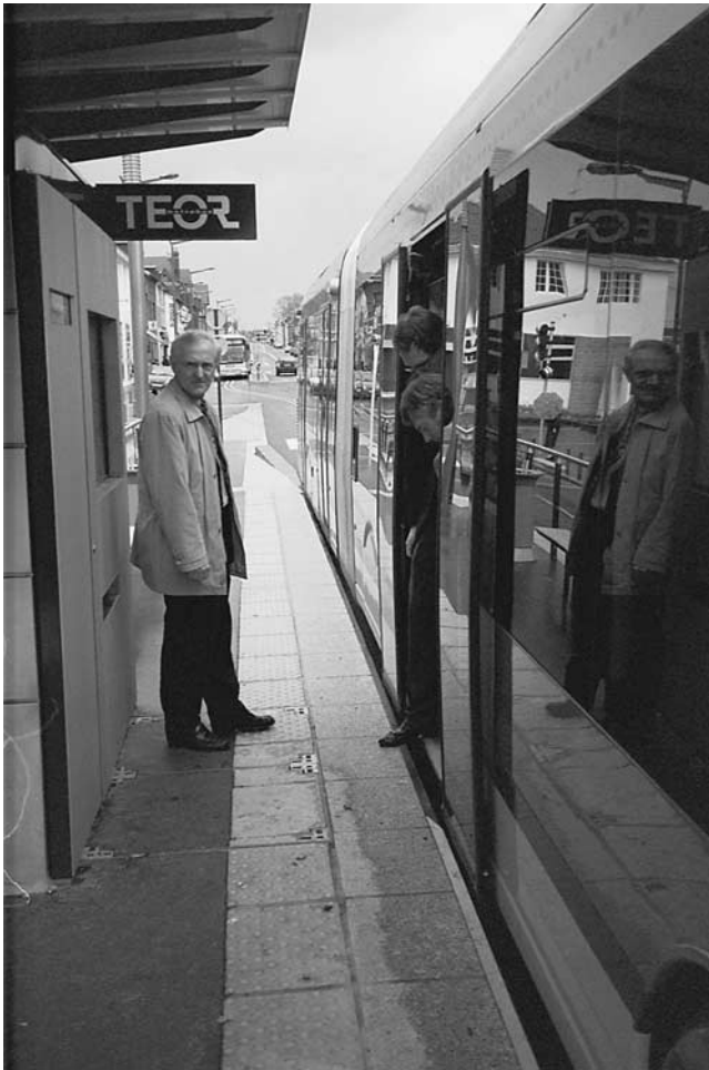
Photo 7-K. Precision docking at stations with a BRT vehicle.
