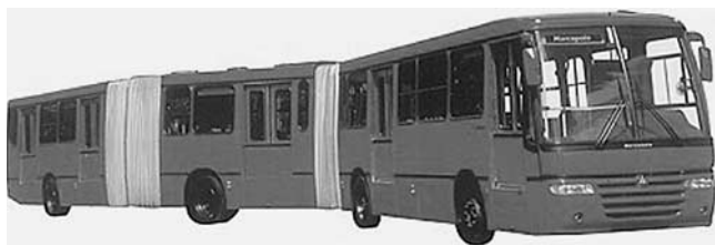
Photo 6-M. Bi-articulated Volvo of Brazil (Marco Polo) high-floor BRT vehicle with boarding/alighting “bridges” in lower part of each door opening (Curitiba, Brazil).
