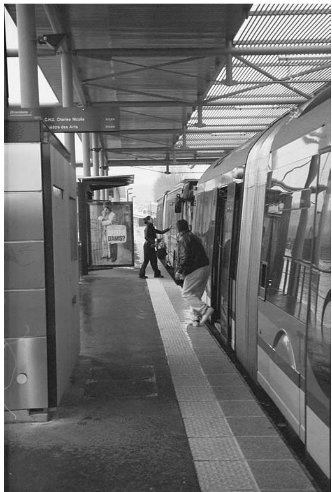
Photo 6-L. No-step boarding and alighting enabled by optical guidance system.
