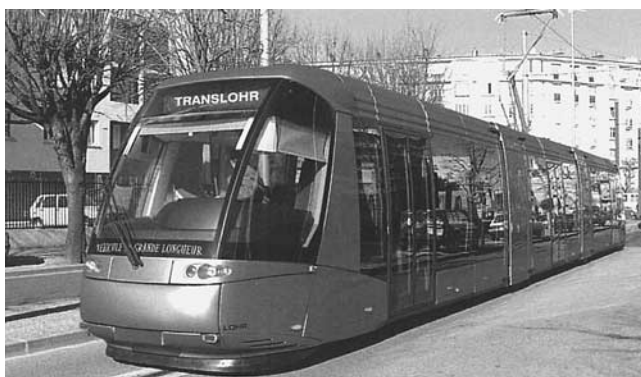
Photo 6-X. 18-meter (60-foot), dual mode, track-guided, modular BRT vehicle.
