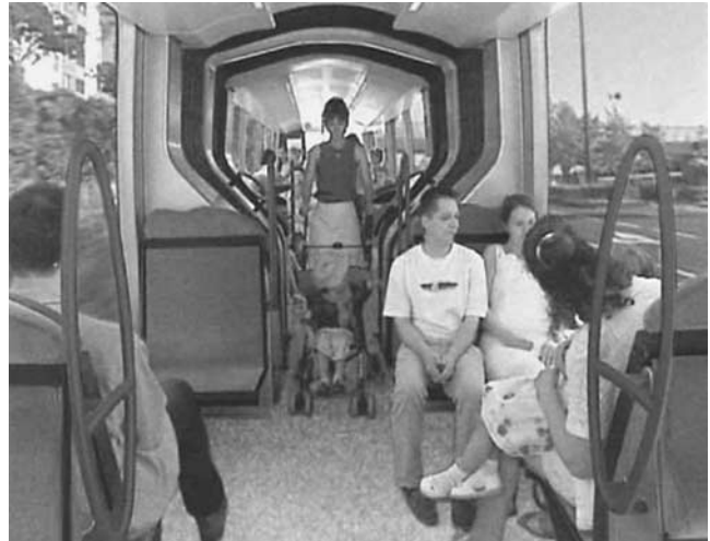
Photo 6-K. Wide, no-step aisle supports circulation and makes it easier to access rear of long, articulated vehicles.
