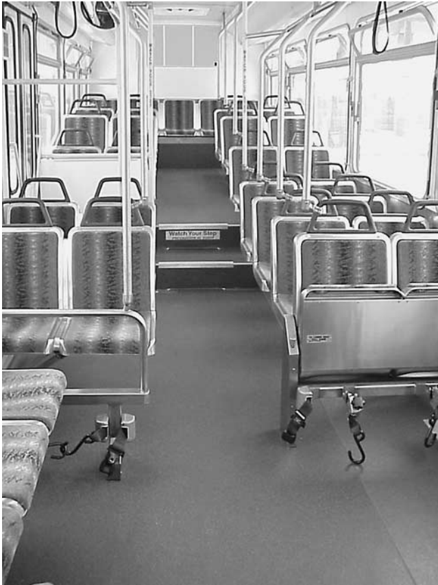
Photo 6-J. 12.2 meter (40-foot), CNG, North American Bus Industries bus with partial (70%) low floor and step up to rear section—Los Angeles Metro Rapid bus.
