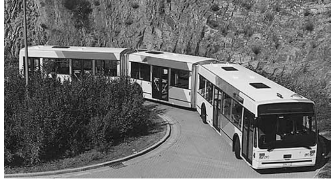
Photo 6-F. Conventional low-floor bus—24-meter (80-foot), double articulated, low-floor.
