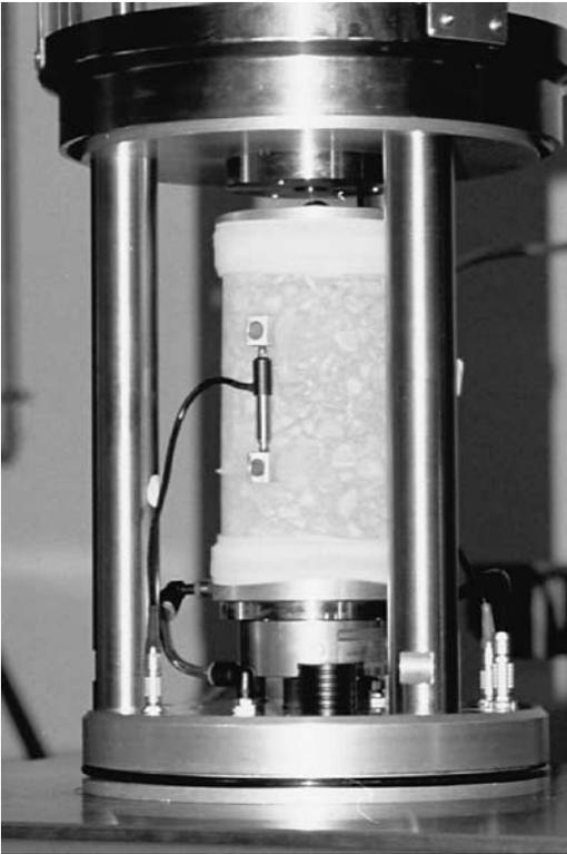
Figure 9. Shedworks dynamic modulus test instrumentation.
