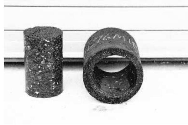
**Figure 4. 100 mm Diameter Core and Waste Ring.**
