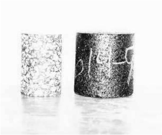
**Figure 6. Final Simple Performance Test Specimen.**
