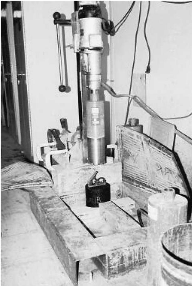
Figure 11. Portable core drilling machine and stand.
