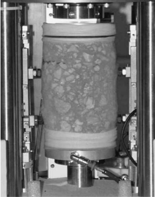
Figure 7. Interlaken dynamic modulus test instrumentation.
