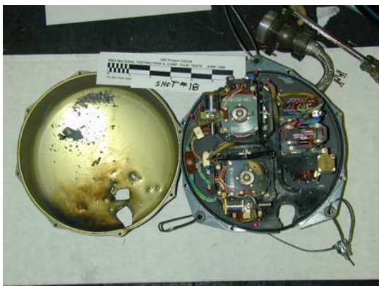
FIGURE 4-1 Damage done by inert fragments to the guidance component of a missile.
