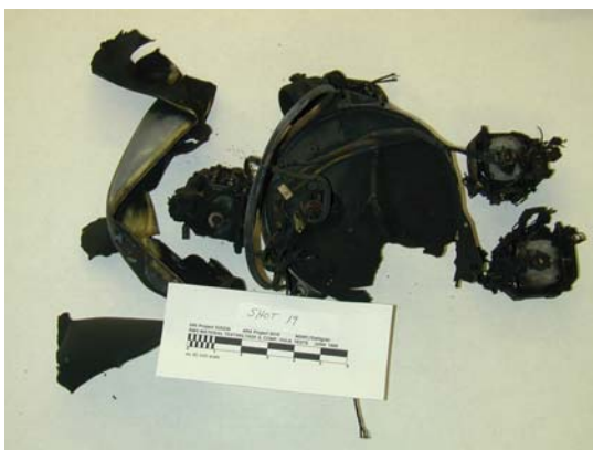
FIGURE 4-2 Damage done by reactive fragments to a guidance component identical to that shown in Figure 4-1.
