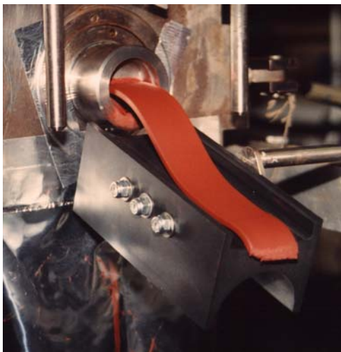
FIGURE 6-5 Slab extrusion using a twin screw extruder.
