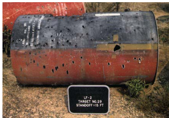
FIGURE 4-3 Damage done to a missile body by a warhead's inert fragments.
