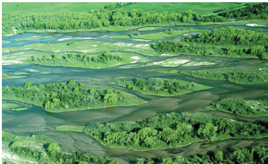
FIGURE 2-3 Channel of Platte River showing its broad, shallow, braided nature. Source: Photograph by W.L. Graf, May 2003.
