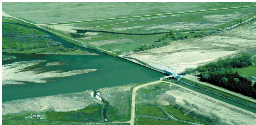
FIGURE 4-5 Johnson-2 diversion on central Platte River, a feature that influences local distribution of flows in river and provides valuable irrigation water for agriculture. Source: Photograph by W.L. Graf, May 2003.
