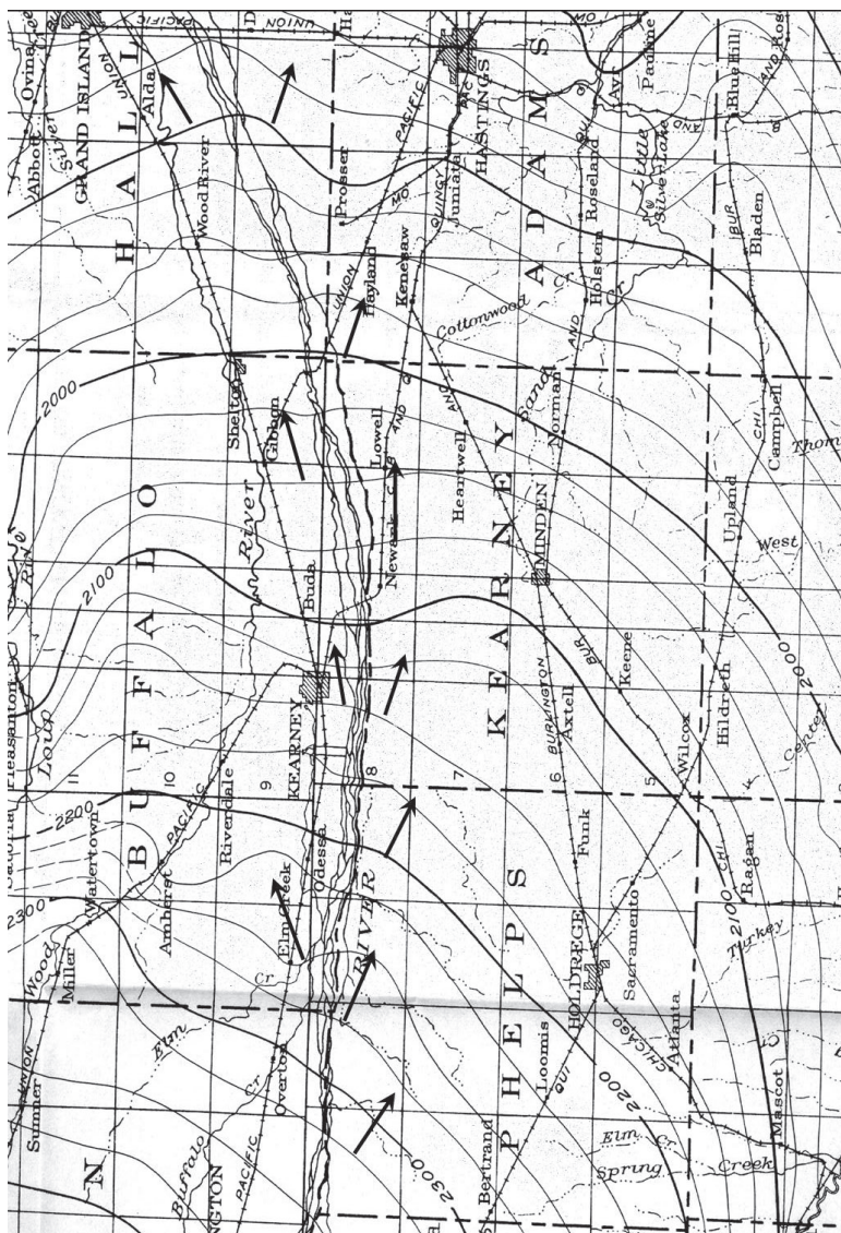
FIGURE 2-15 Map of elevation of groundwater table in 1931 shown as contour surface. Water flows down-gradient and generally eastward and southeastward. Compare with Figure 2-16. Source: Adapted from Woodward 2003.
