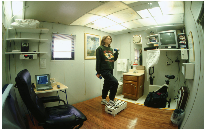
FIGURE D-13 The whole-room indirect calorimeter at Vanderbilt University.
