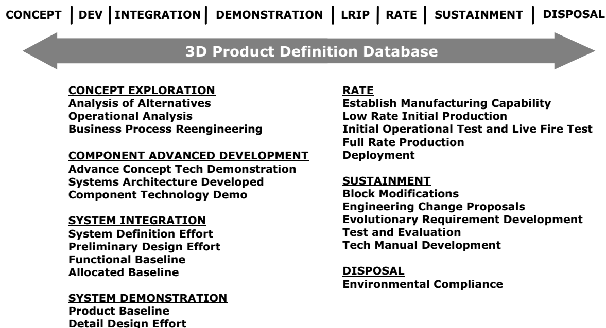
FIGURE 3-4 Life-cycle phases expanded into the eight indicated at the top of the figure. Source: A. Adlam, U.S. Army, "TACOM Overview," presented to the Committee on Bridging Design and Manufacturing, National Research Council, Washington, D.C., June 25-26, 2003.
