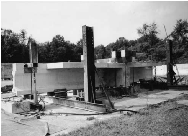
Figure 7. Test set-up for the stub girder specimens.
