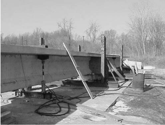
Figure B-15. Full-size specimen with loading cylinders.
