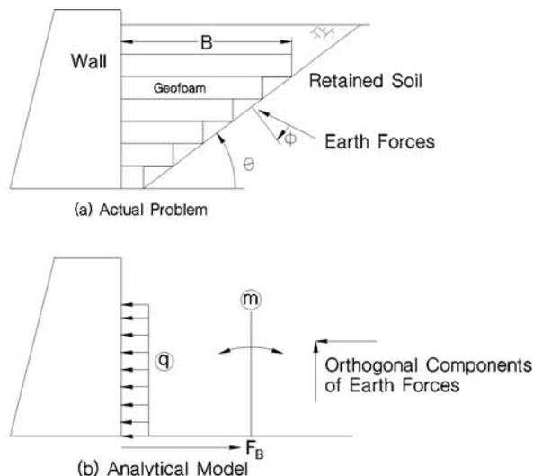
Figure 50. Seismic load components on a wall. ( $F_B$  = resisting force against sliding and  $m$  = seismic moment.)
