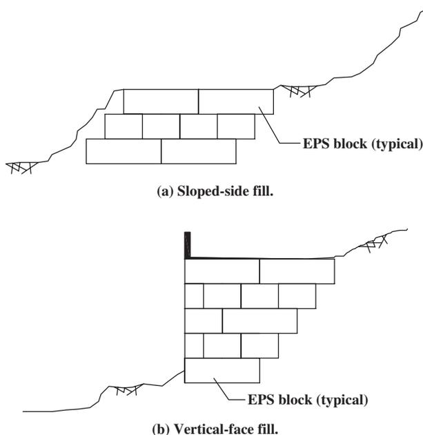
Figure 2. Typical EPS-block geofoam applications involving side-hill fills (2).
