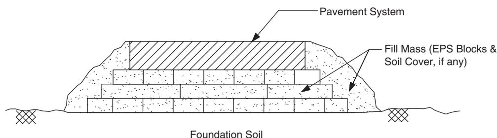
Figure 3. Major components of an EPS-block geofam embankment.
