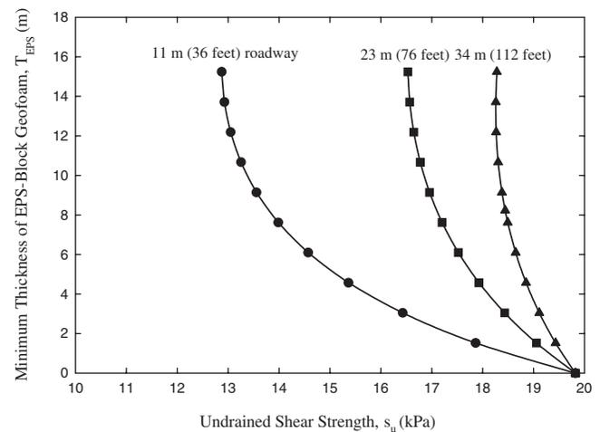
Figure 5. Design chart for obtaining the minimum thickness or height of geofam,  $T_{EPS}$ , for a factor of safety of 3 against external bearing capacity failure of a geofam embankment.
