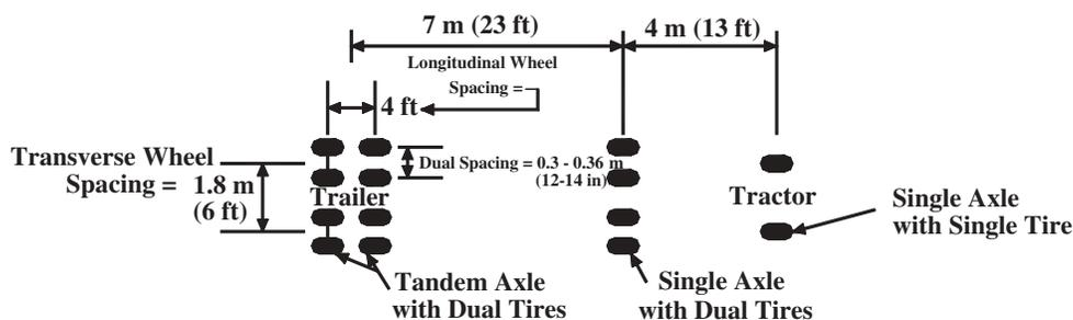
Figure 40. Wheel configuration of a typical semitrailer truck (14).
