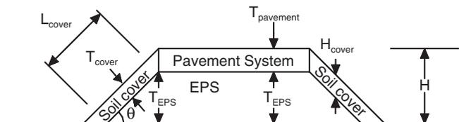
Figure 21. Variables for the weight induced by the soil cover. ( $L_{cover}$  = length of soil cover on the side of the embankment,  $T_{cover}$  = perpendicular thickness of the soil cover, and  $H_{cover}$  = vertical thickness of the soil cover.)
