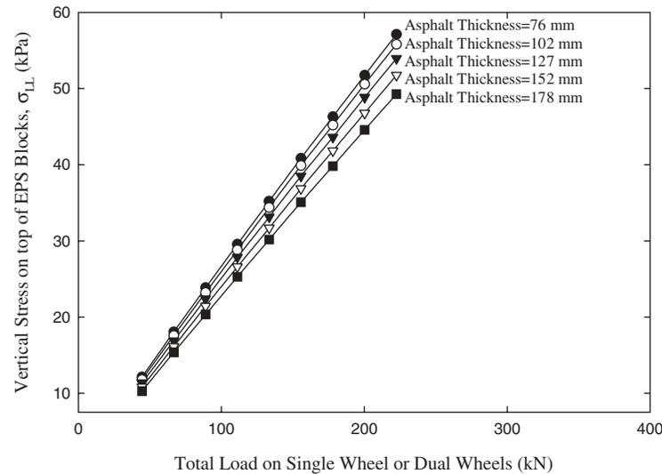
Figure 43. Vertical stress on top of the EPS blocks,  $\sigma_{LL}$ , due to traffic loads on top of a 610-mm (24-in.) asphalt concrete pavement system with a 102-mm (4-in.) concrete separation layer between the pavement system and EPS blocks.
