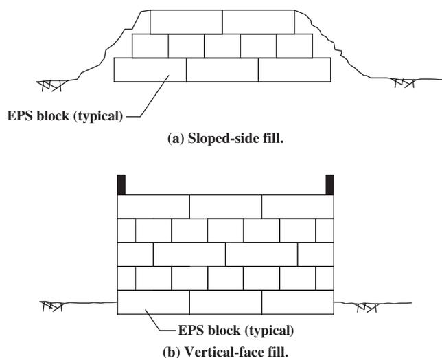
Figure 1. Typical EPS-block geofoam applications involving embankments (2).
