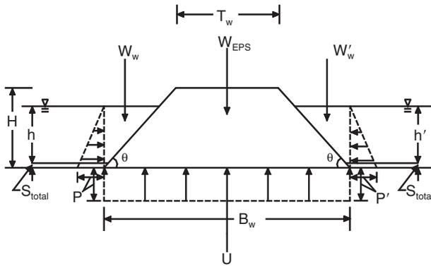
Figure 20. Variables for determining hydrostatic uplift for the case of water equal on both sides of the embankment. (*P* = pressure exerted on the side of the embankment and *U* = uplift pressure acting on the base of the embankment.)
