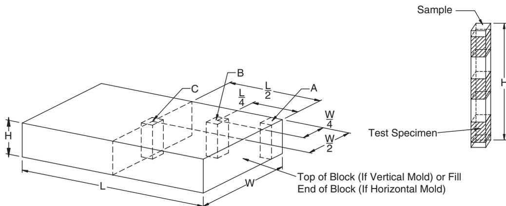
Figure 1. Recommended block sampling and test specimens.
