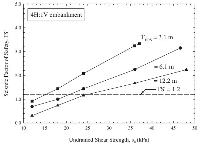
Figure 13. Seismic external slope stability design chart for trapezoidal embankments with a six-lane roadway with a total road width of 34 m (112 ft) and a  $k_h$  of 0.05.
