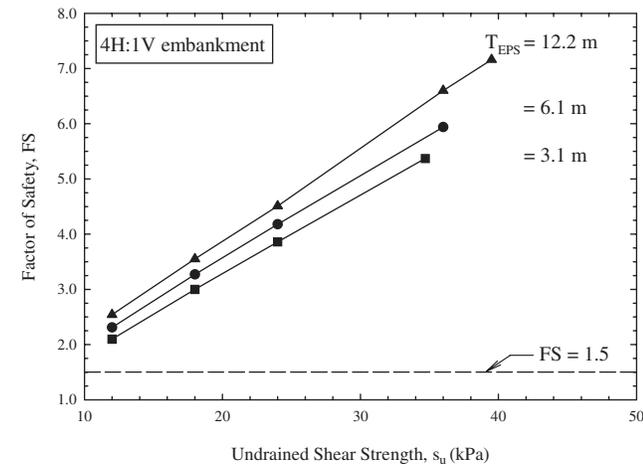
Figure 7. Static external slope stability design chart for trapezoidal embankments with a two-lane roadway with a total road width of 11 m (36 ft).
