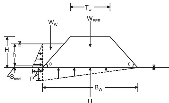
Figure 26. Variable for determining hydrostatic uplift analysis for the case of water on one side of the embankment only. ( $P$  = pressure exerted on the side of the embankment and  $U$  = uplift pressure acting on the base of the embankment.)
