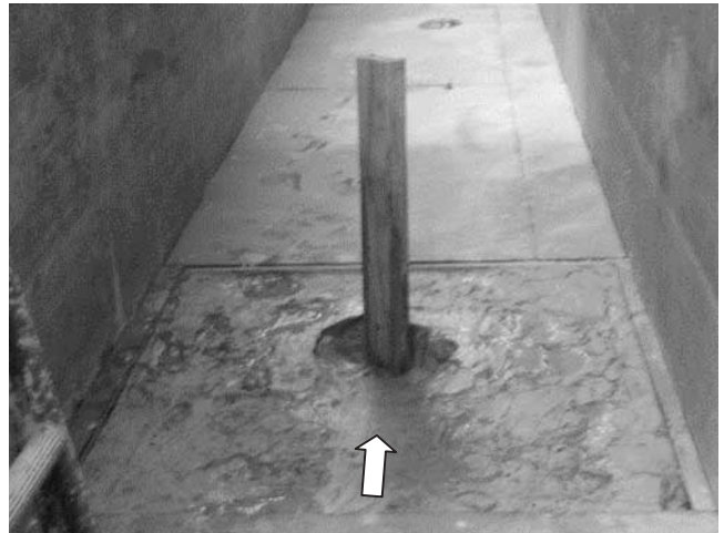
Figure A17 Scour Hole in Test At-6—Back View.
