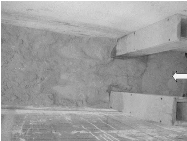
Figure A31 Scour Hole in Contraction Scour Test 13— Back View.
