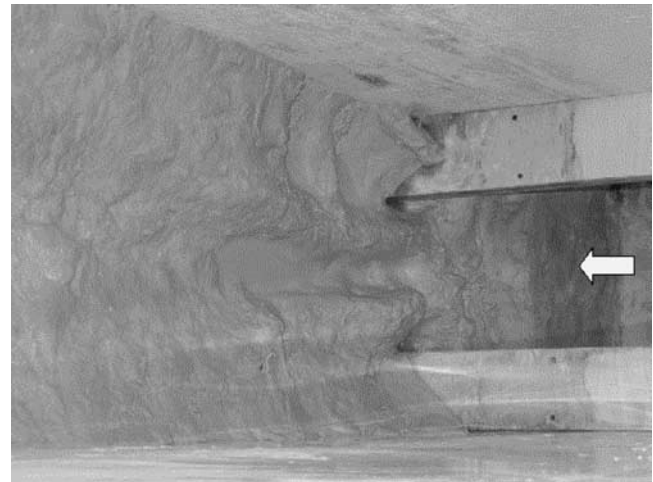
Figure A33 Scour Hole in Contraction Scour Test 14.
