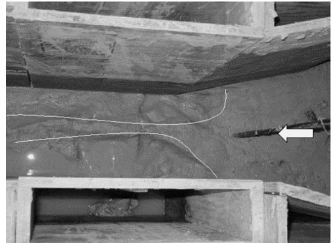
Figure A28 Scour Hole in Contraction Scour Test 9.
