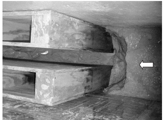
Figure A22 Scour Hole in Contraction Scour Test 1.
