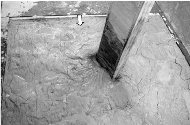
Figure A14 Scour Hole in Test At-1—Back View.
