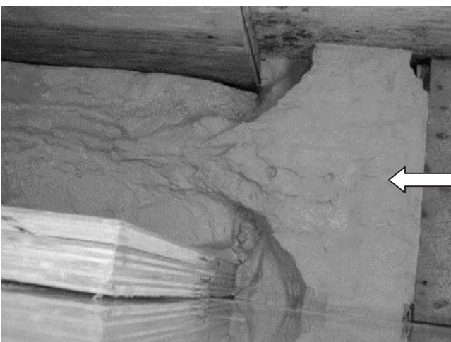
Figure A26 Scour Hole in Contraction Scour Test 3.
