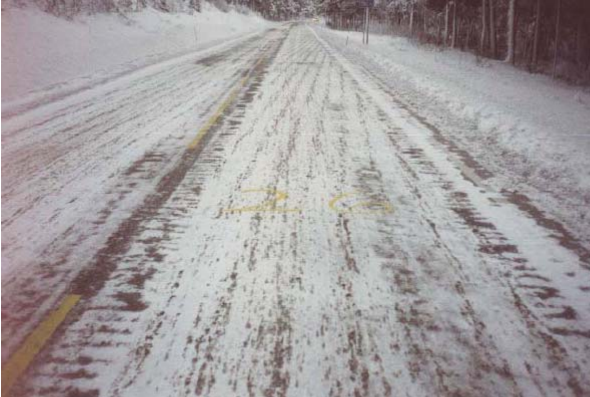
FIGURE 9 Test field strewn with warm wetted sand January 18, 2001. Picture taken January 22.
