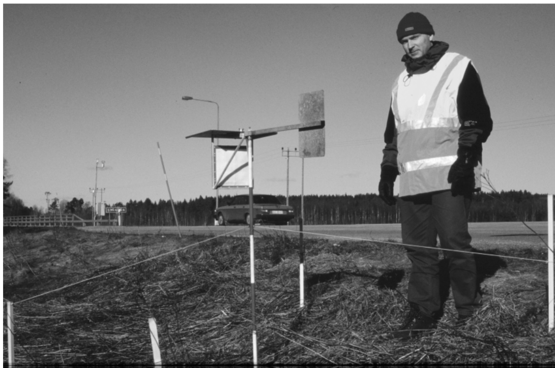
FIGURE 3 Salt vane at the Vimmerby field site.
