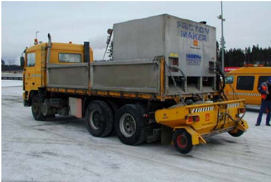
FIGURE 2 Swedish prototype for warm wetted sand.
