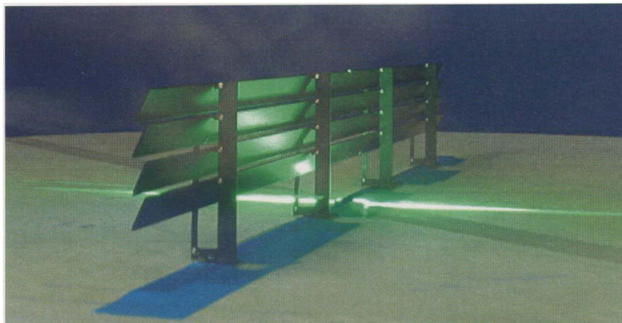
FIGURE 2 Model blower snow fence (11 cm high).
