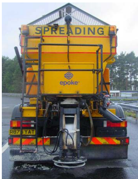
FIGURE 1 A typical prewetting salt vehicle used in the UK.
