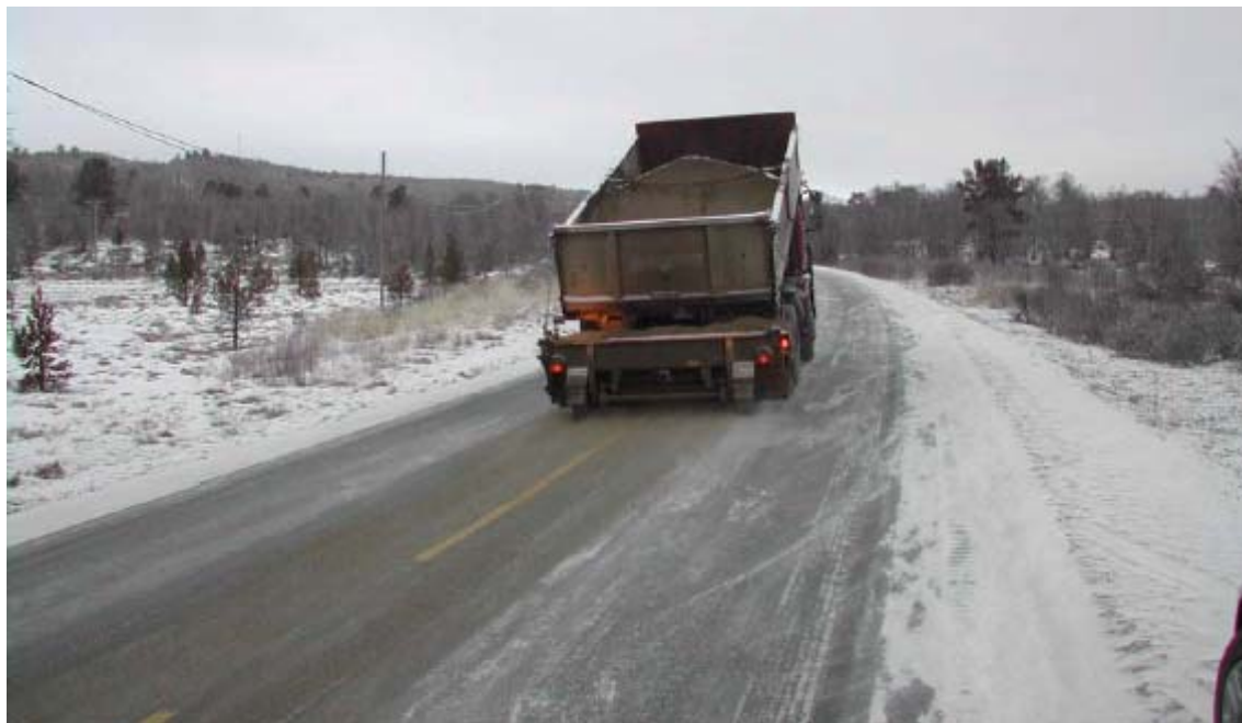
FIGURE 1 Traditional sanding method with dry sand.
