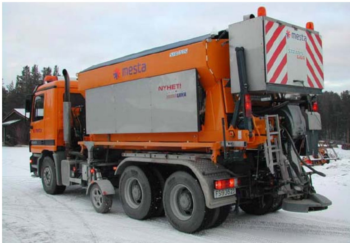
FIGURE 14 Warm wetted sand spreader with friction device.
