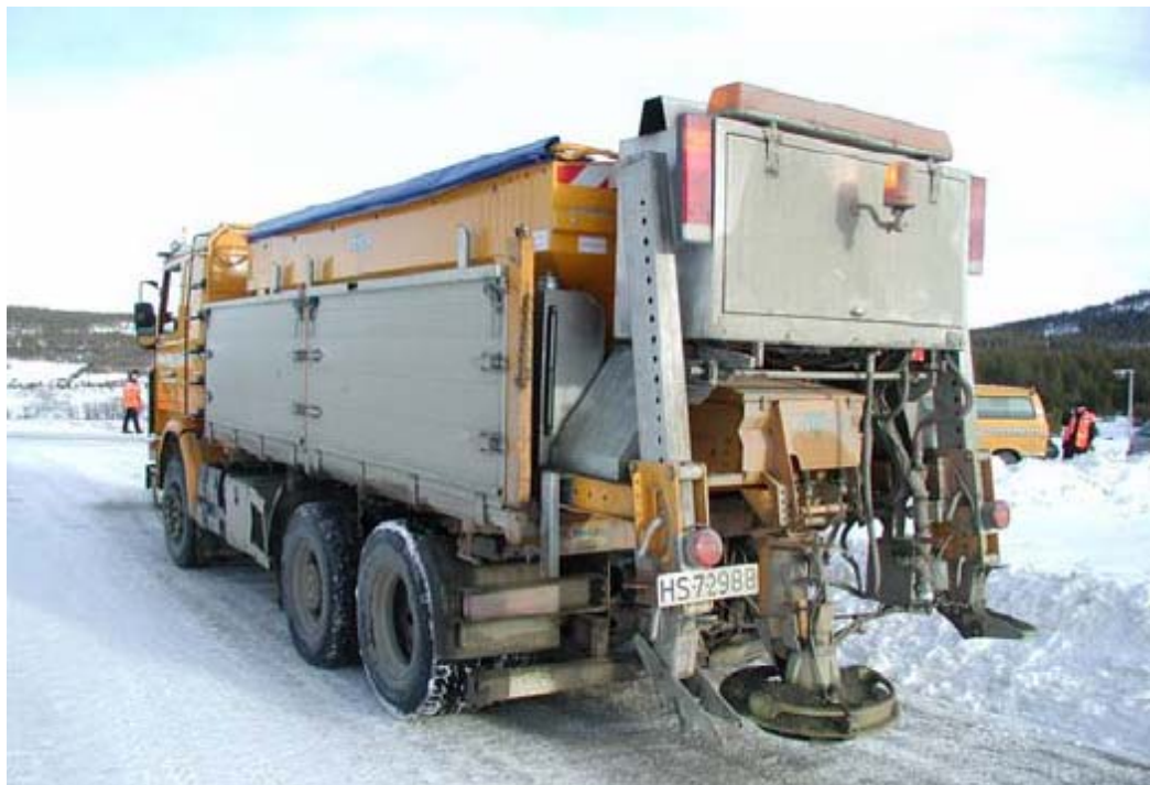
FIGURE 3 New concept for warm wetted sand spreader.
