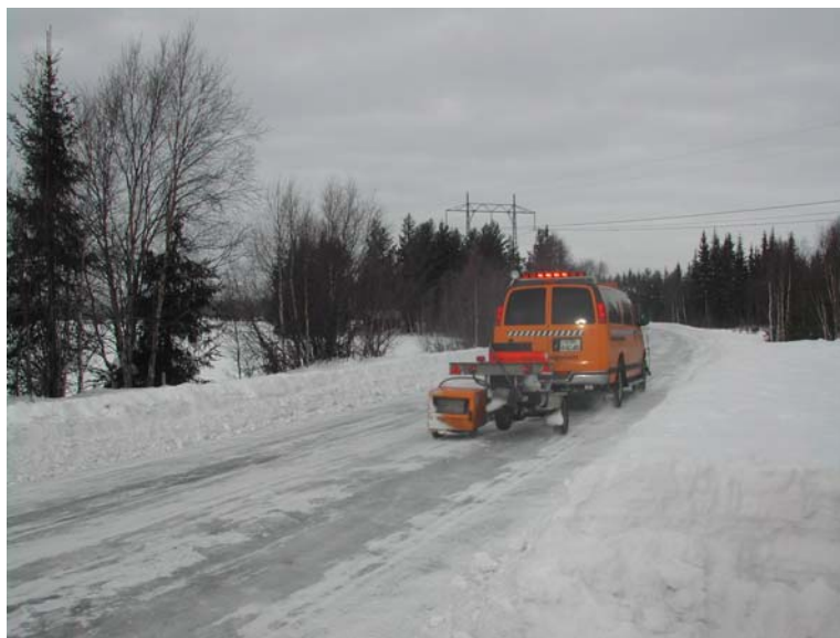
FIGURE 6 Roar friction trailer.
