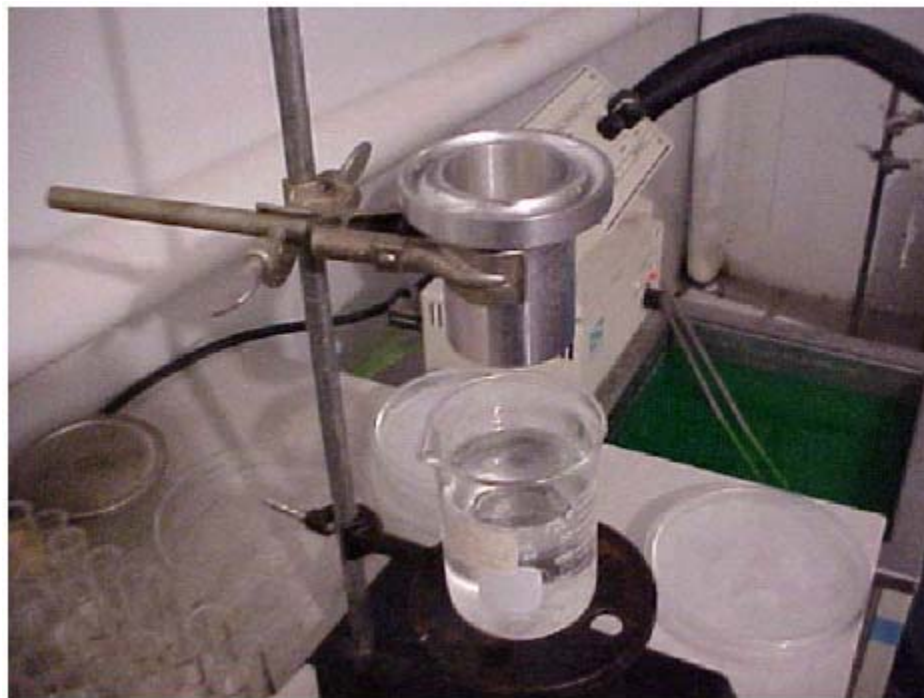
FIGURE 1 Viscosity measured with a Ford #2 cup viscometer.
