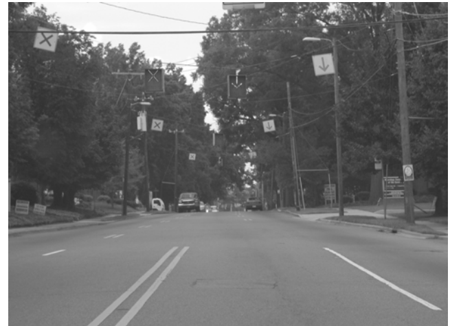
FIGURE 9 Simple reversible lane transition, Charlotte, N.C.
