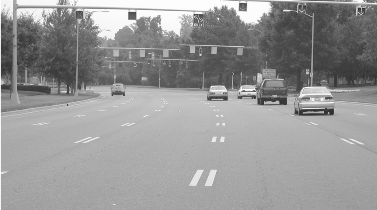
FIGURE 42 Tyvola Road—lane-use control signals, Charlotte, N.C.
