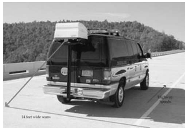
FIGURE 8 Scanning laser [Courtesy: Mandli Communications (41)].
