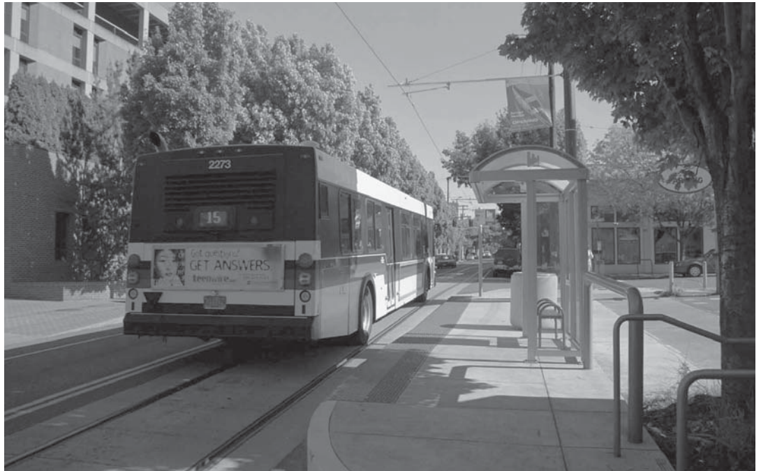
A Portland, Oregon, bus stops in the traffic lane to load and unload riders, called on-line loading. The clearance time—the amount of time needed for a bus to clear the stop—differs between on-line and off-line loading. In off-line loading, buses stop out of traffic and must wait for a suitable gap in traffic before re-entering.
